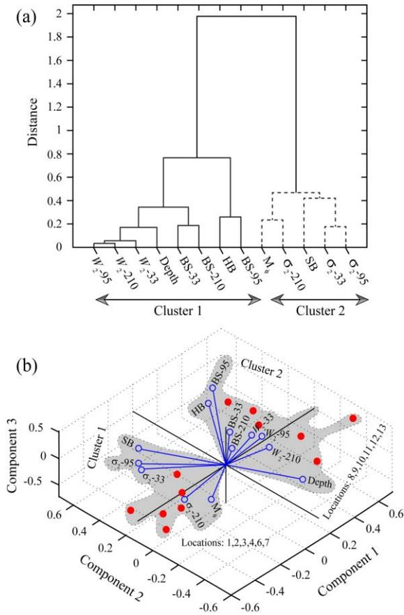
Fig. 4—The dendrogram in panel (a) and biplot of PCA (b) illustrates the location wise clustering of measured and derived parameters. The acronym BS, SB, HB denotes backscatter, soft body and hard body benthic macro-fauna respectively.
