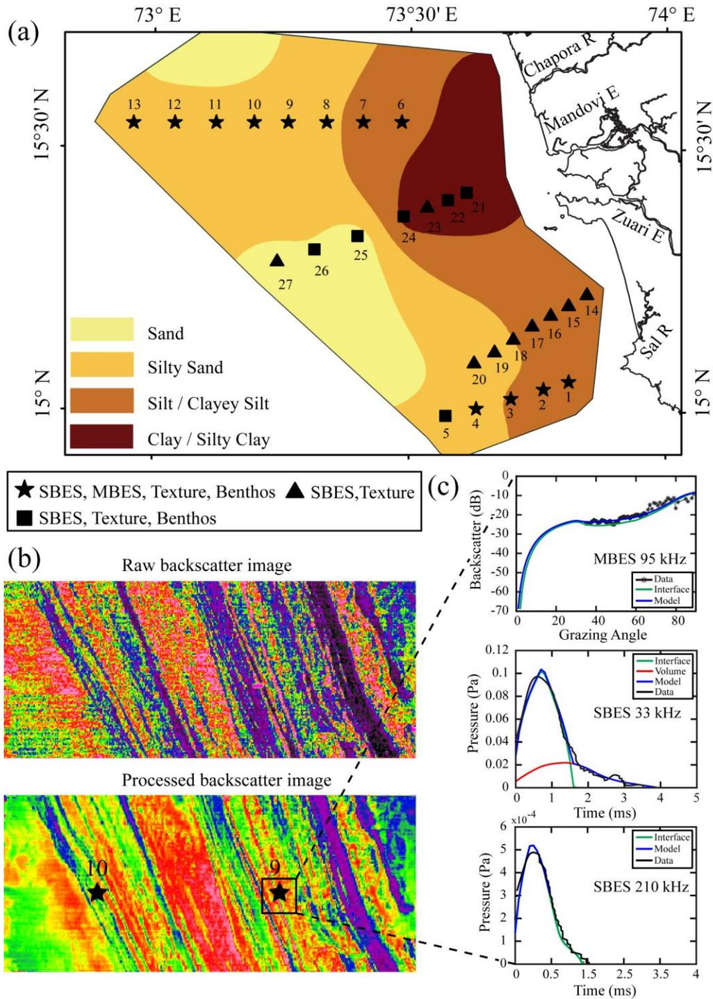
Fig. 1(a)–Shows the study area and type of data collected (modified from Haris *et al.*<sup>6</sup>). Panel (b) depicts the application of PROBASI algorithm to process EM 1002 MBES backscatter data. The processed SBES and MBES backscatter data used to carry out the inversion modeling are presented in (c). The inversion results are analyzed with the sediment texture and benthic macro-faunal abundance obtained at the same locations.
