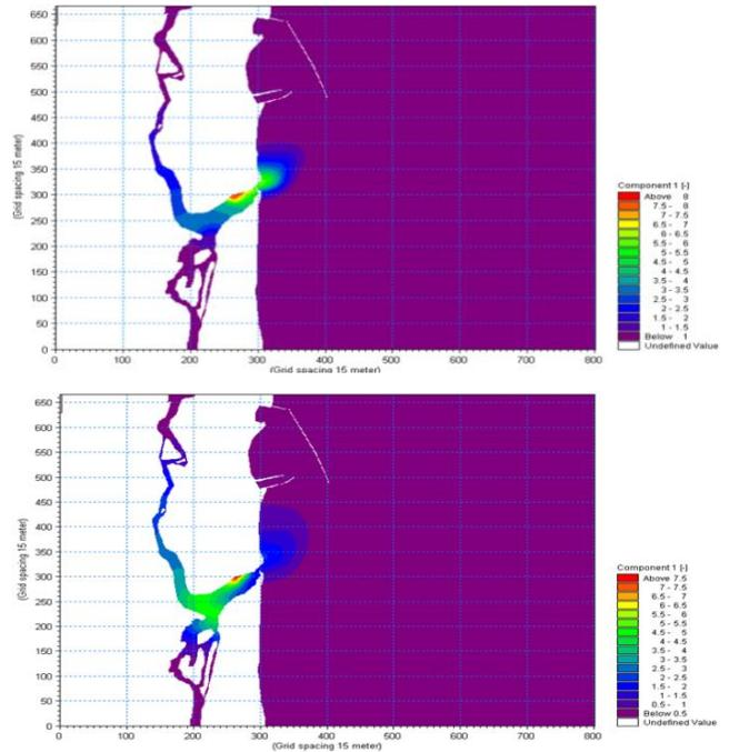
Fig. 11—Thermal Dispersion from Low Tide to High Tide
