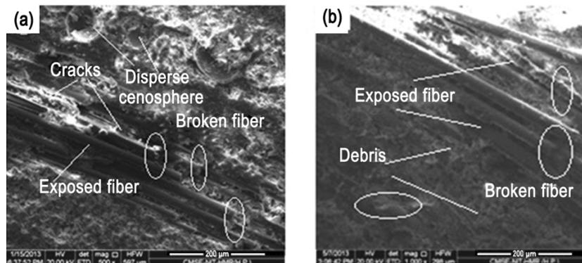
Fig. 8 – SEM pictures of the worn surface of composite specimens ( $C_3$ ) at applied normal load 70 N and sliding speed 5.7 m/s (a) under dry sliding condition and (b) under water lubrication sliding conditions
