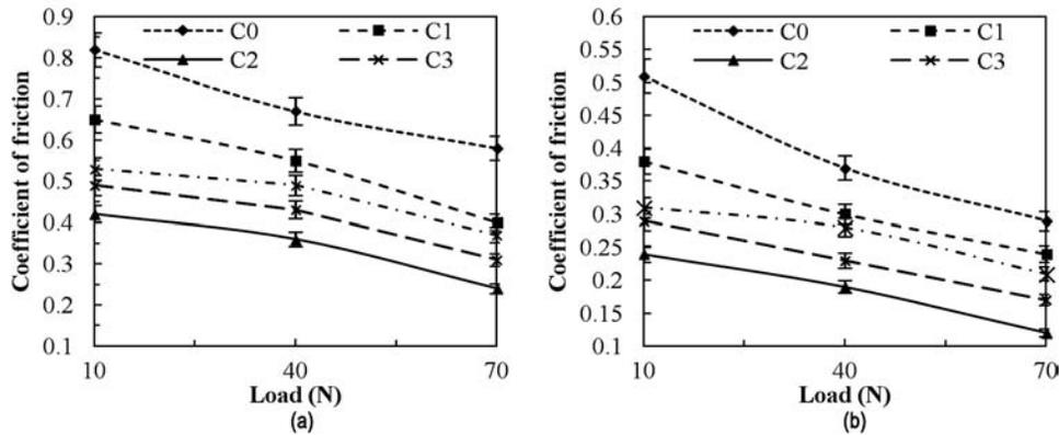
Fig. 1 – Variation of coefficient of friction of the glass fiber reinforced vinylester composites at 5.7 m/s (a) under dry conditions and (b) under water lubricated conditions
