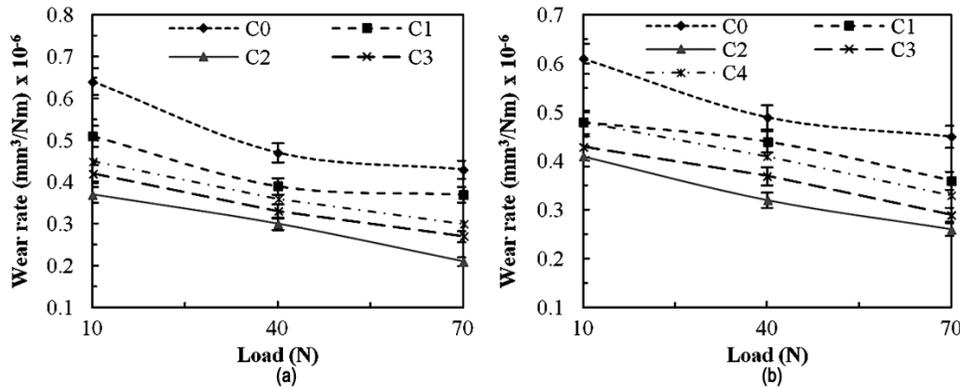
Fig. 3 – Variation of specific wear rate of the glass fiber reinforced vinylester composites at 5.7 m/s of (a) under dry sliding conditions and (b) under water sliding conditions
