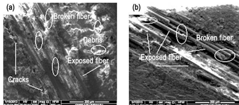
Fig. 6 – SEM pictures of the worn surface of composite specimens ( $C_1$ ) at applied normal load 70 N and sliding speed 5.7 m/s (a) under dry sliding condition and (b) under water lubrication sliding conditions
