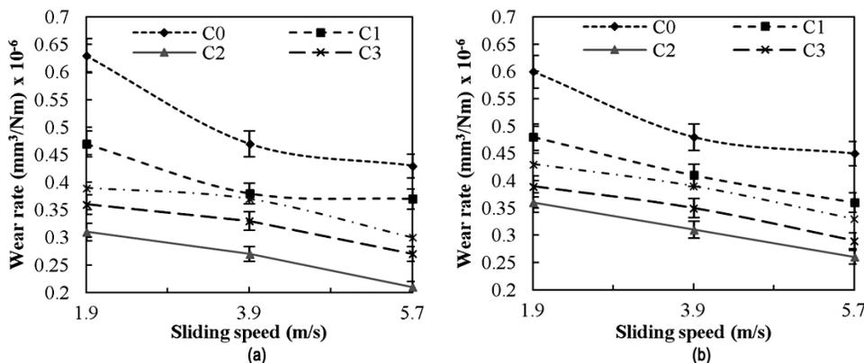
Fig. 4 – Variation of specific wear rate of the glass fiber reinforced vinylester composites at 70 N of (a) under dry sliding conditions and (b) under water sliding conditions
