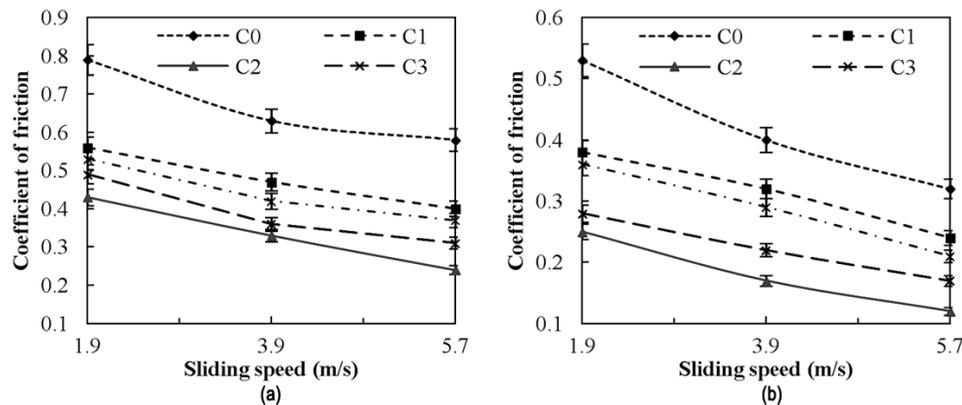
Fig. 2 – Variation of coefficient of friction of the glass fiber reinforced vinylester composites at normal load 70 N of (a) under dry conditions and (b) under water lubricated conditions
