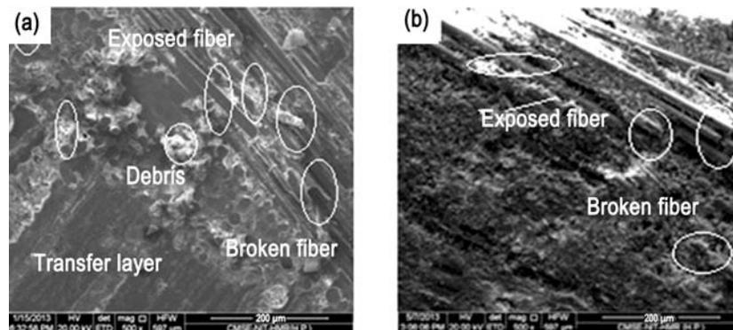
Fig. 7 – SEM pictures of the worn surface of composite specimens ( $C_2$ ) at applied normal load 70 N and sliding speed 5.7 m/s (a) under dry sliding condition and (b) under water lubrication sliding conditions
