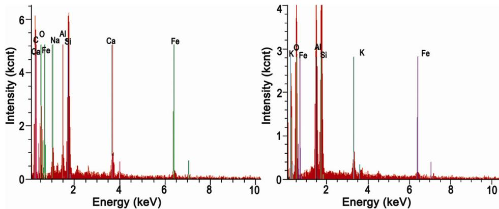
Fig. 10 – EDS spectrograph of cenosphere filled (10 wt%) glass fiber reinforced vinylester composites at applied normal load 70 N and sliding speed 5.7 m/s (a) under dry sliding condition and (b) under water lubricated sliding condition
