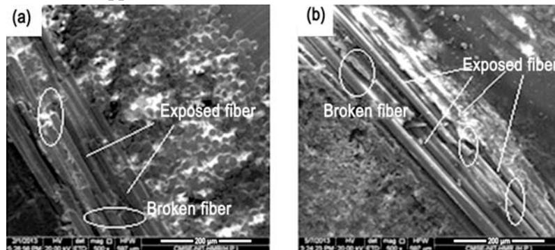
Fig. 5 – SEM pictures of the worn surface of composite specimens ( $C_0$ ) at applied normal load 70 N and sliding speed 5.7 m/s (a) under dry sliding condition and (b) under water lubrication sliding conditions
