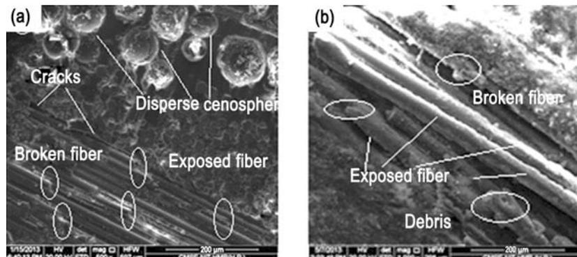
Fig. 9 – SEM pictures of the worn surface of composite specimens ( $C_4$ ) at applied normal load 70 N and sliding speed 5.7 m/s (a) under dry sliding condition and (b) under water lubrication sliding conditions
