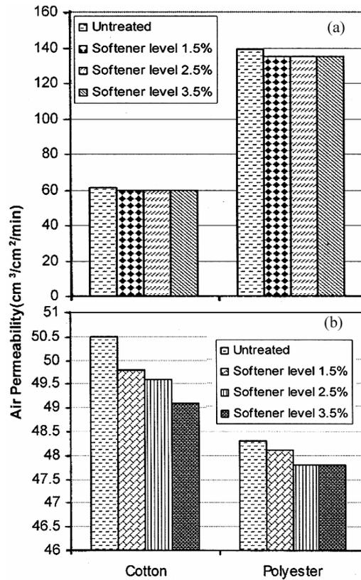
Fig. 2—Mean scores of air permeability by fabric softener treatments for (a) coarser count and (b) finer count cotton and polyester fabrics
