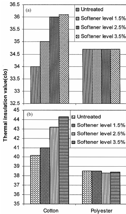
Fig. 1—Mean scores of thermal insulation values by fabric softener treatments for (a) coarser count and (b) finer count cotton and polyester fabrics
