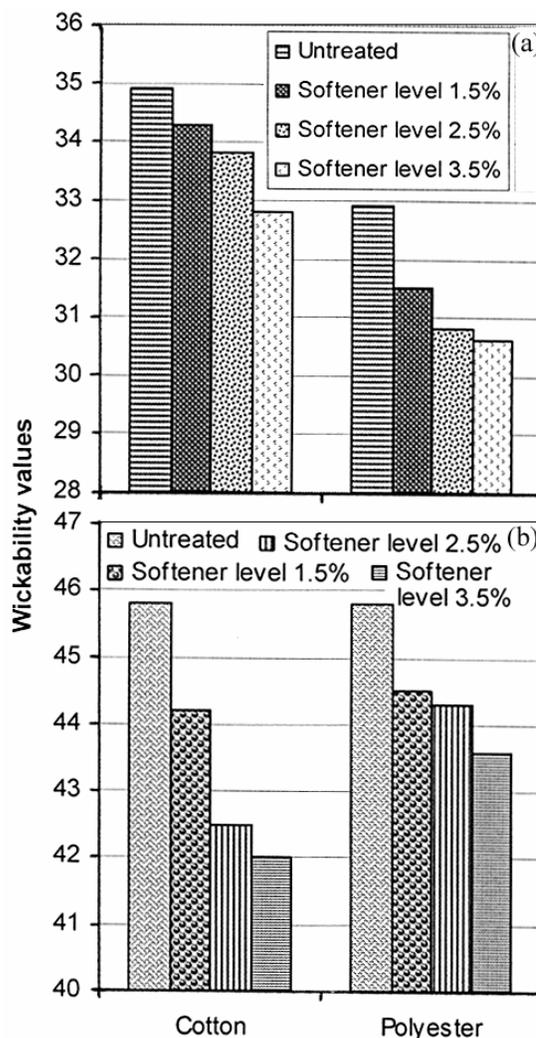
Fig. 3—Mean scores of wickability by fabric softener treatments for (a) coarser count and (b) finer count cotton and polyester fabrics
