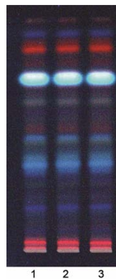
Fig. 2—TLC profile of Yavānyādi cūrṇa observed under 366 nm; Track 1: Batch 01, Track 2: Batch 02, Track 3: Batch 03
