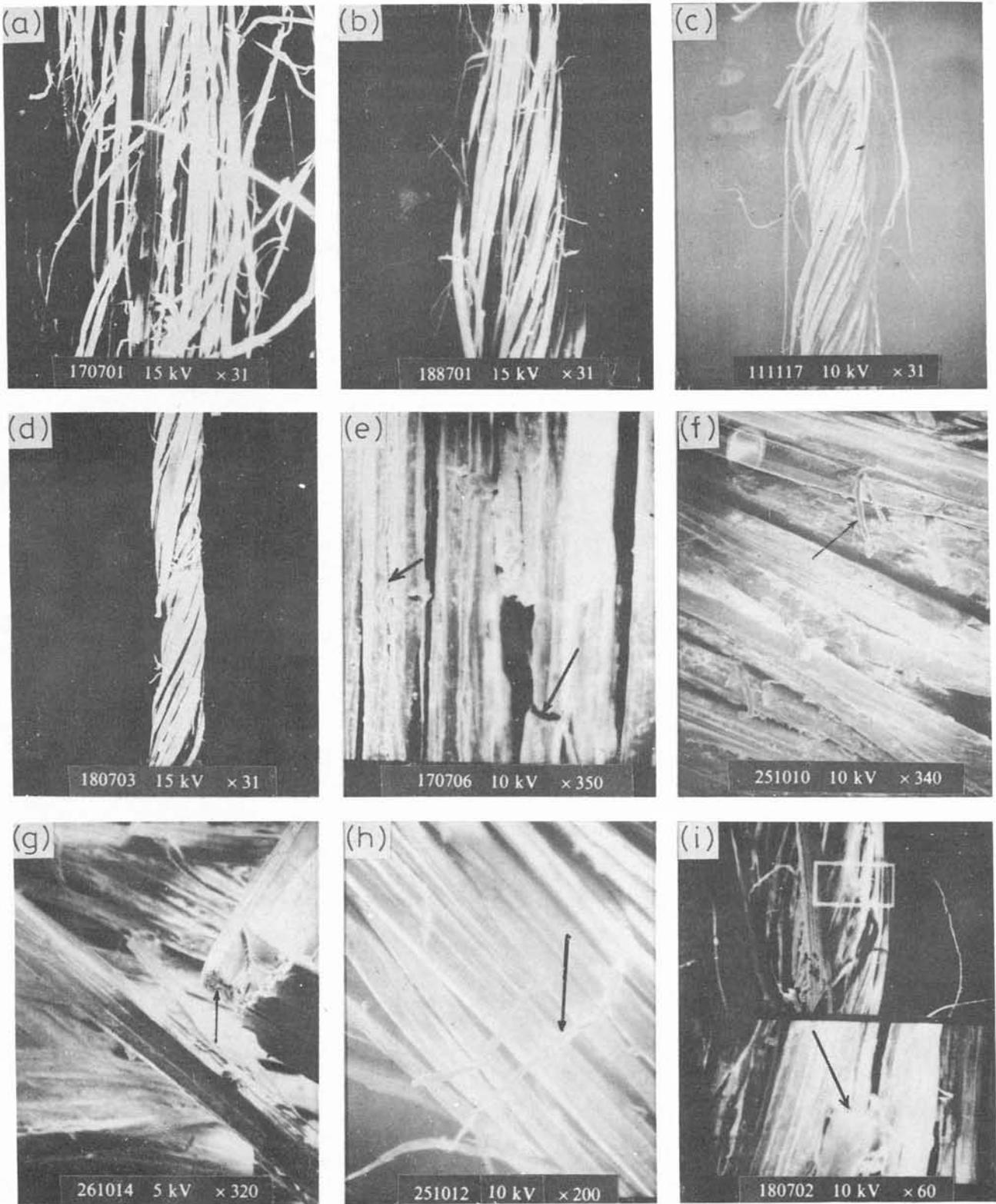
Fig. 1— Electron micrographs of jute yarn of 276 tex [(a) Twist 3 TPI, × 31; (b) twist 4.40, × 31; (c) twist 5 TPI, × 31; (d) twist 6 TPI, × 31; (e) twist 4.40 TPI, × 350; (f) twist 5 TPI, × 340; (g) twist 6 TPI, × 320; (h) twist 6 TPI, × 200; and (i) twist 6 TPI, × 60 — Fractured end of the filament at the twisting zone (× 300)]
