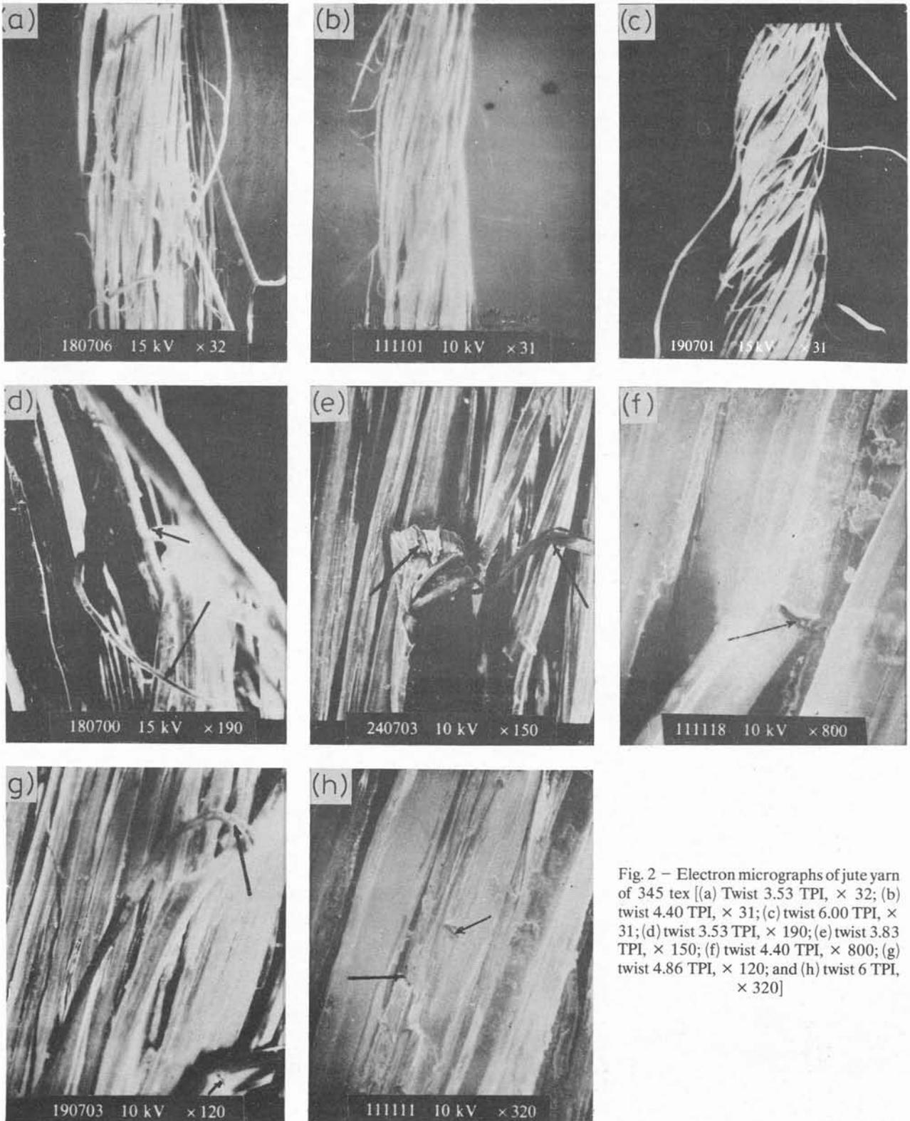
Fig. 2 - Electron micrographs of jute yarn of 345 tex [(a) Twist 3.53 TPI, × 32; (b) twist 4.40 TPI, × 31; (c) twist 6.00 TPI, × 31; (d) twist 3.53 TPI, × 190; (e) twist 3.83 TPI, × 150; (f) twist 4.40 TPI, × 800; (g) twist 4.86 TPI, × 120; and (h) twist 6 TPI, × 320]
