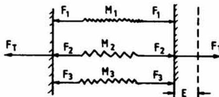
Fig. 1—Stress distribution in yarn of warp sheet
