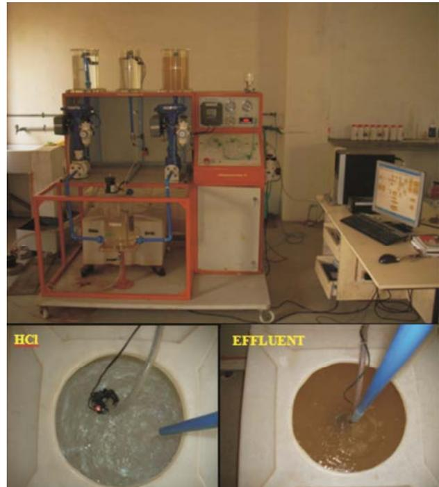
Fig. 2 — pH system with industrial effluent
