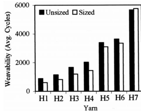
Fig. 5—Weavability of 49 tex unsized core dref yarns
