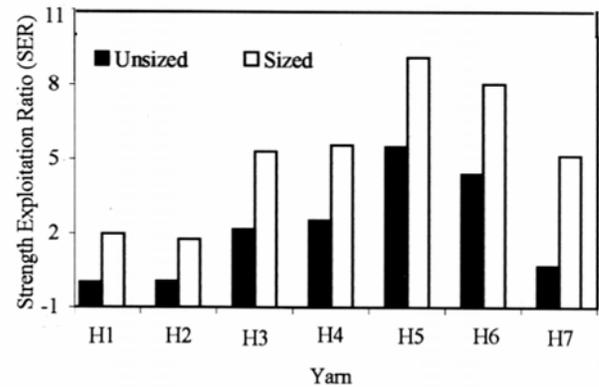
Fig. 2—Strength exploitation ratio of 49 tex core-spun dref yarns
