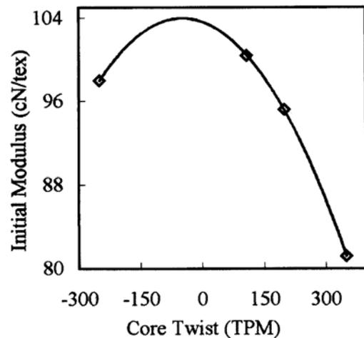
Fig. 3—Effect of core filament twist on initial modulus of 49 tex core dref yarns
