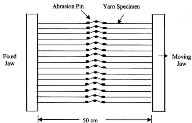
Fig. 1—Working principle of webtester
