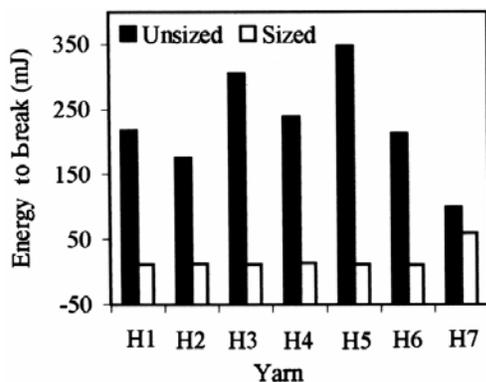
Fig. 4—Energy-to-break of 49 tex core dref yarns
