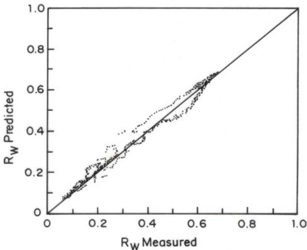
Fig. 3—Reflectance of the sample immersed in water ( $R_w$ ) predicted from equation plotted against the measured values
