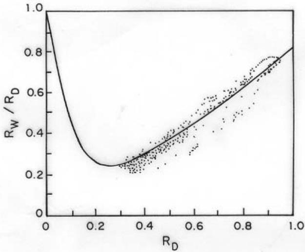
Fig. 2 — Ratio of the reflectance of the sample immersed in water ( $R_w$ ) to that of the dry one ( $R_d$ ) plotted against the reflectance of the dry sample
