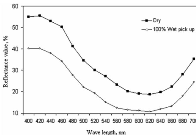
Fig. 1 — Effect of moisture content on reflectance values of fabric dyed with Direct Blue 77
