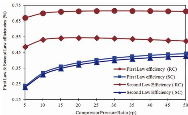
Fig. 1—Effect of Compressor Pressure Ratio ( $r_p$ ) on First law and Second Law Efficiency of regeneration cycle (RC) and simple cycle (SC) [TIT=1900 K,  $T_0=298$  K]
