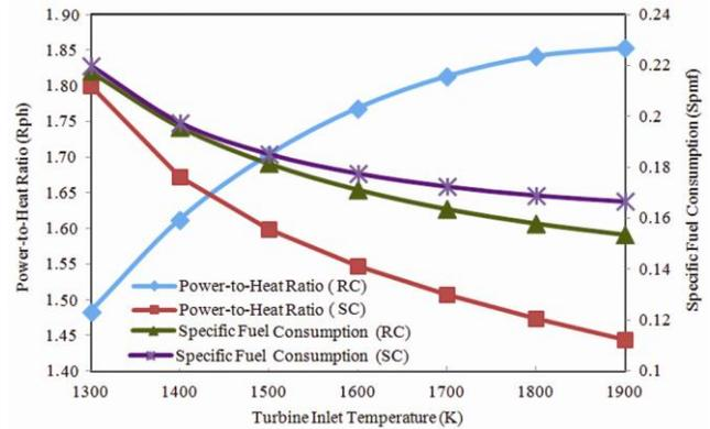
Fig. 3—Effect of Turbine Inlet Temperature (K) on Power-to-heat Ratio ( $R_{ph}$ ) and Specific Fuel Consumption (sfc) of Regeneration cycle (RC) and Simple Cycle (SC)
