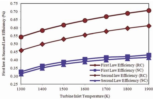
Fig. 2—Effect of Turbine Inlet Temperature (K) on First Law efficiency, Second Law Efficiency of Regeneration cycle (RC) at  $r_p = 20$  and Simple Cycle (SC) at  $r_p = 40$
