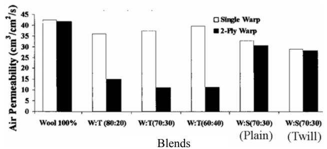
Fig. 6 — Air permeability of single and 2-ply yarn woven worsted fabrics
