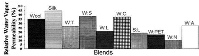
Fig. 9 — Effect of blend composition on relative water vapour permeability
