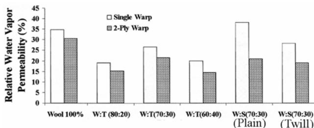
Fig. 10 — Relative water vapour permeability of single and 2-ply warp woven worsted fabrics
