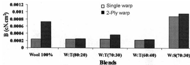
Fig. 3 — Bending rigidity (B) of single and equivalent 2-ply yarns
