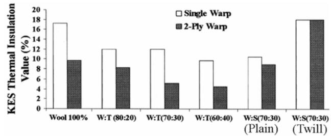
Fig. 8 — Thermal insulation of single and 2-ply warp woven worsted fabrics
