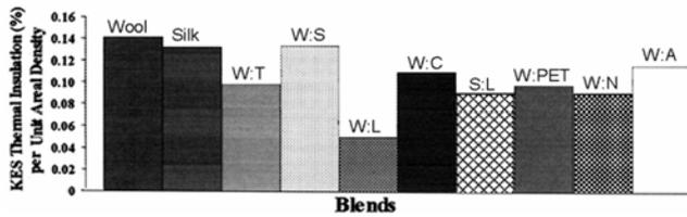
Fig. 7 — Thermal insulation per unit areal density for different worsted blends
