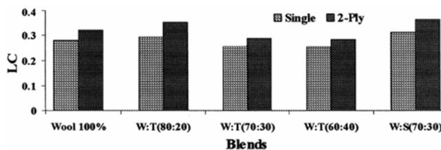
Fig. 4 — Compressibility (LC) of single and equivalent 2-ply yarns
