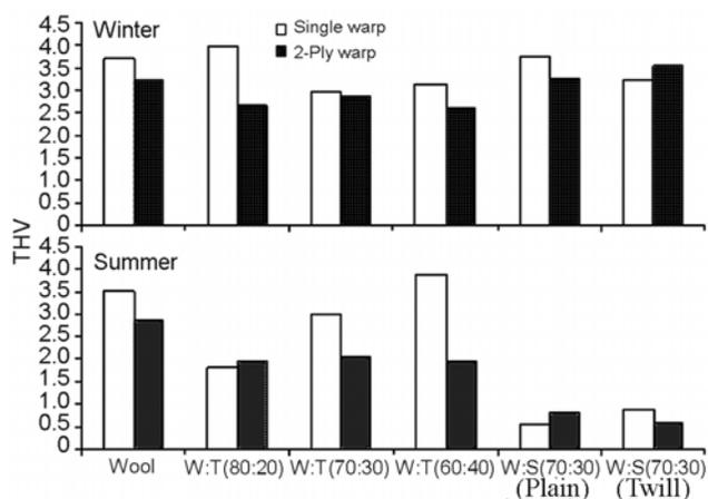
Fig. 2 — THV for single and 2-ply yarn woven worsted fabrics
