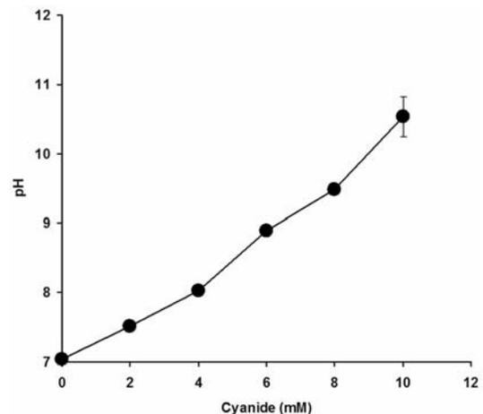
Fig. 2—Effect of cyanide on pH of reaction mixture. [Values represent mean ± SE of 3 replicates]
