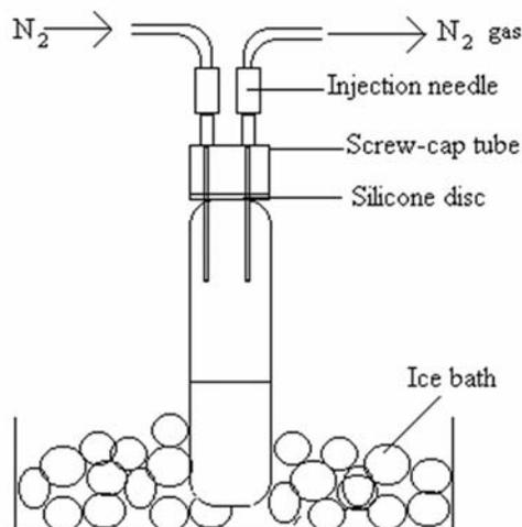
Fig. 1—Procedure for maintenance of anaerobic conditions for molybdenum reduction.
