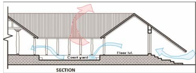
Fig. 7—Courtyard, minimum openings and projected eaves reduce the solar heat gain and regulate the air flow through the building.
