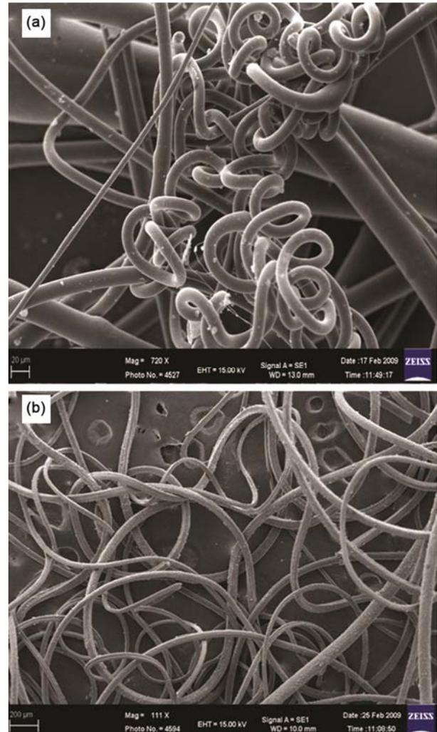
Fig. 2(a,b)—SEM images of PC-1.5% MWNT fibers
