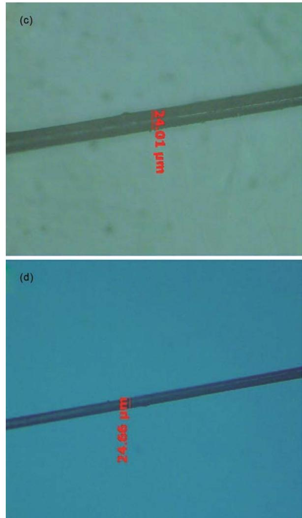
Fig. 1(c,d)—Optical micrographs of PC-1.5% MWNT fiber
