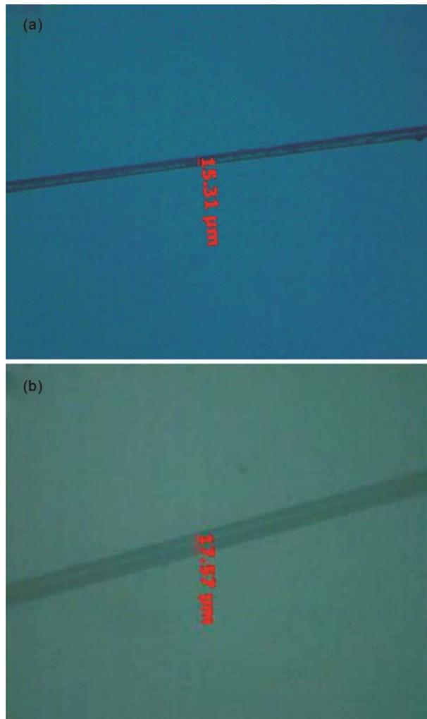
Fig. 1(a,b)—Optical micrographs of PC-1% MWNT fiber
