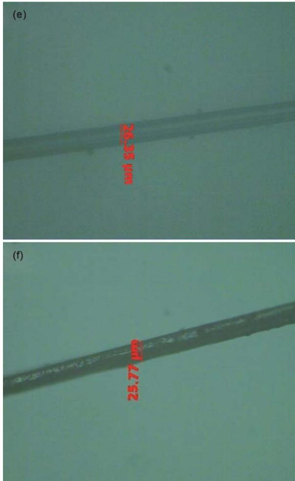
Fig. 1(e,f)—Optical micrographs of PC-2% MWNT fiber
