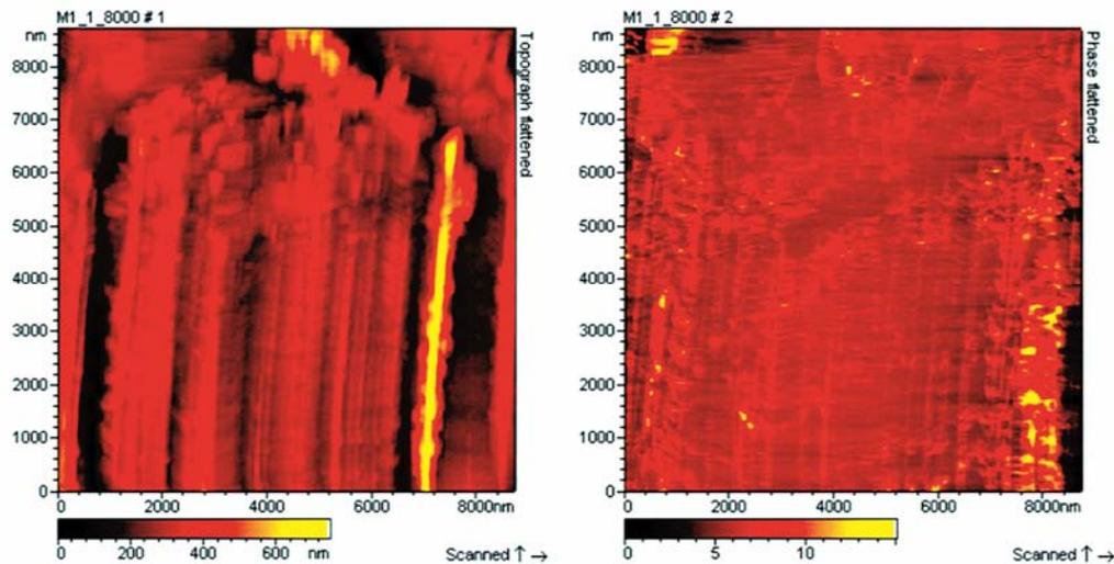
Fig. 3—AFM of single PC-1.5% MWNT fiber
