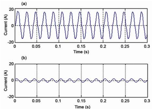
Fig. 10—Neutral current before and after installing SHAPF
