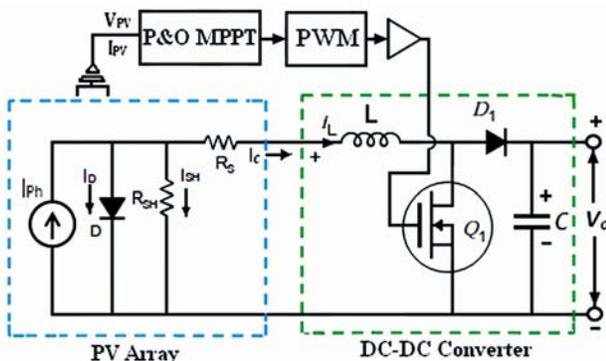
Fig. 2—Topology of PV operated DC-DC boost converter
