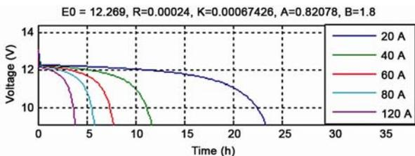
Fig. 12—Discharge characteristics of the battery for various output currents
