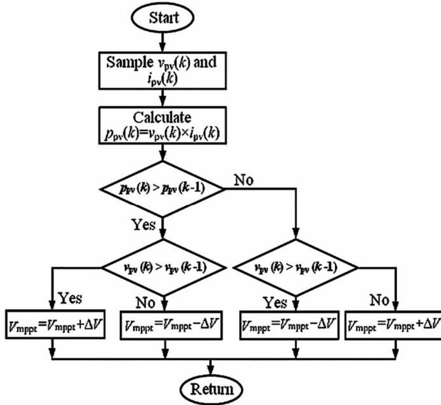
Fig. 3—Flowchart of P&O MPPT algorithm
