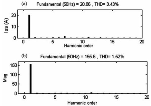
Fig. 9—THD level of source current and load voltage after compensation in phase-'a'
