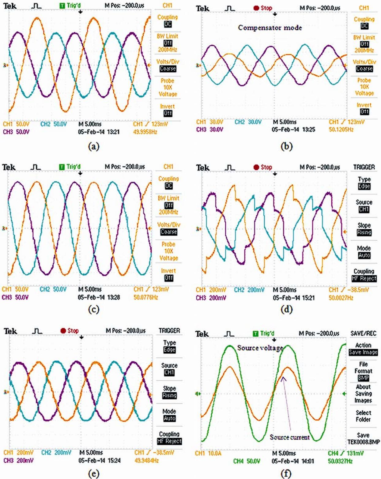
Fig. 13—Experimental results under balanced voltages with unbalanced loads: (a) source voltages ( $V_{sabc}$ ) before compensation, (b) injected voltage, (c) Load voltage ( $V_{labc}$ ) after compensation, (d) load currents ( $i_{labc}$ ), (e) source currents ( $i_{sabc}$ ) after compensation and (f) source voltage ( $V_{sa}$ ) superimposed by the source current ( $i_{sa}$ )
