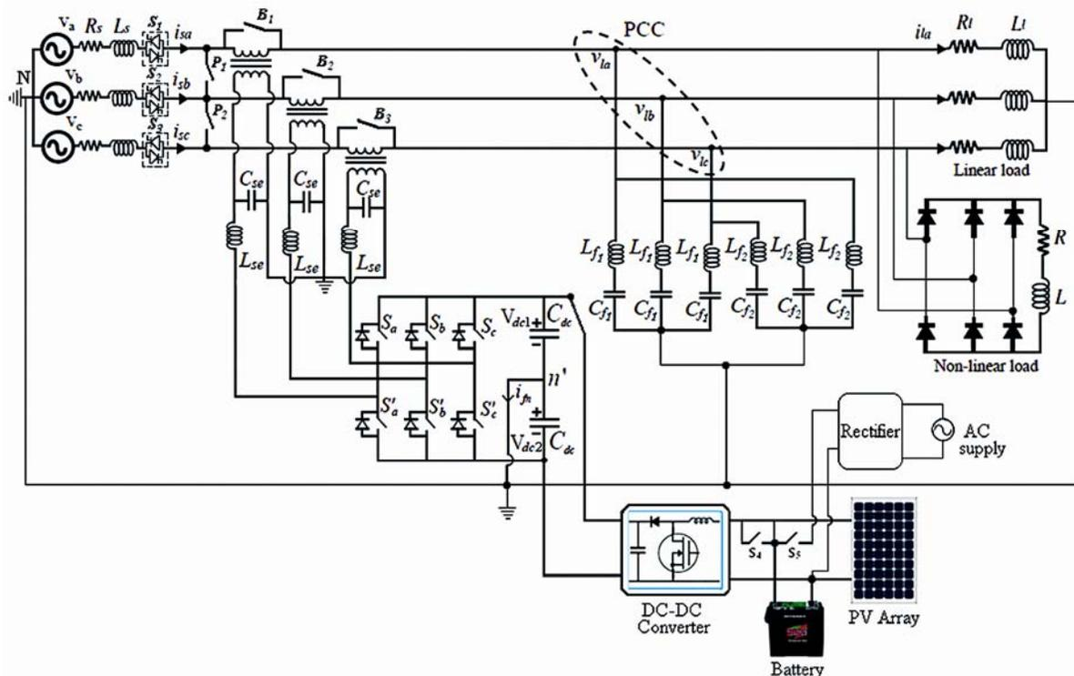
Fig. 1—PV based series active filter with shunt passive filter topology
