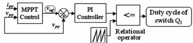
Fig. 4—Control structure of P&O MPPT
