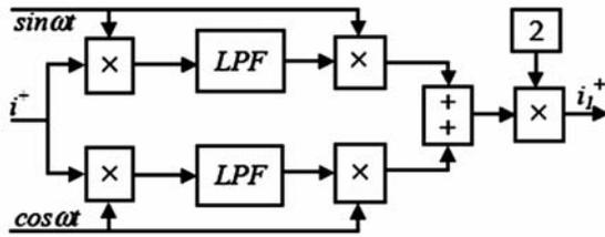
Fig. 6—Fundamental component calculation block
