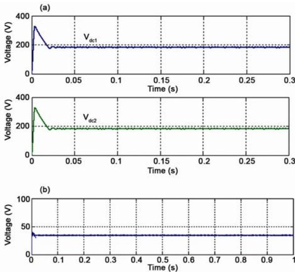
Fig. 11—DC-link capacitor voltage and PV array output voltage
