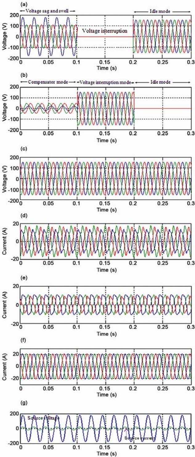
Fig. 8—Simulation results under balanced voltages with unbalanced loads: (a) source voltages ( $V_{sabc}$ ) before compensation, (b) injected voltage, (c) load voltage ( $V_{labc}$ ) after compensation, (d) load currents ( $i_{labc}$ ), (e) active filter currents ( $i_{fabc}$ ), (f) source currents ( $i_{sabc}$ ) and (g) source voltage ( $V_{sa}$ ) superimposed by the source current ( $i_{sa}$ )
