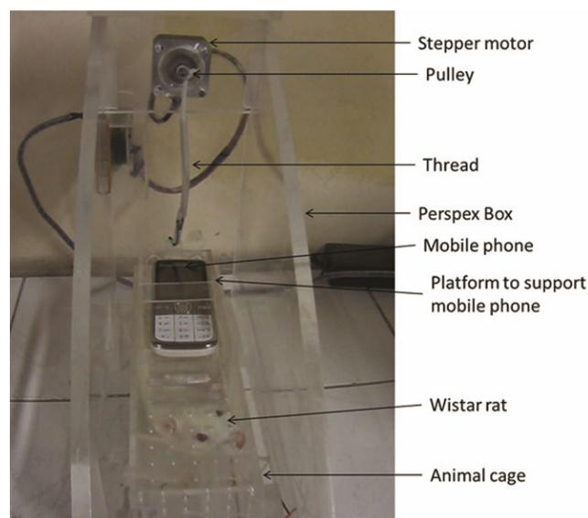
Fig. 1—Exposure set up of 3G mobile phone on Perspex animal holding cage (length: 55 cm, width: 17.5 cm, height: 15 cm). One end of platform supporting the mobile phone was tied to a string and the other end was fixed to the animal cage by a hinge. The string was attached to a pulley, movement of which was controlled by a stepper motor. The stepper motor was programmed to be controlled by a personal computer
