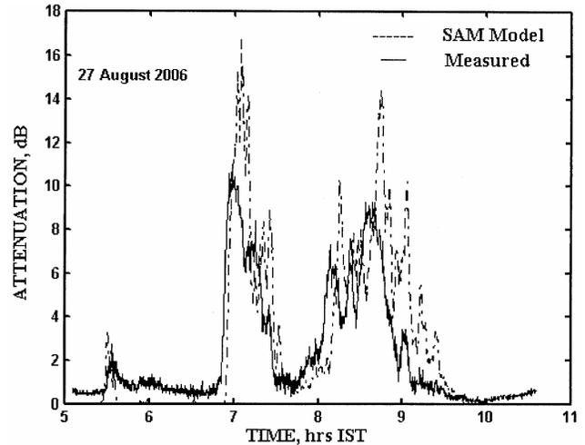
Fig. 4—Comparison between measured attenuation and SAM model generated values during a rain event
