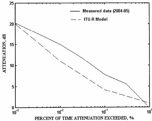
Fig. 3—Cumulative distributions Ku-band attenuation over an earth-space path for Kolkata obtained experimentally during June 2004–June 2005 and from ITU-R models
