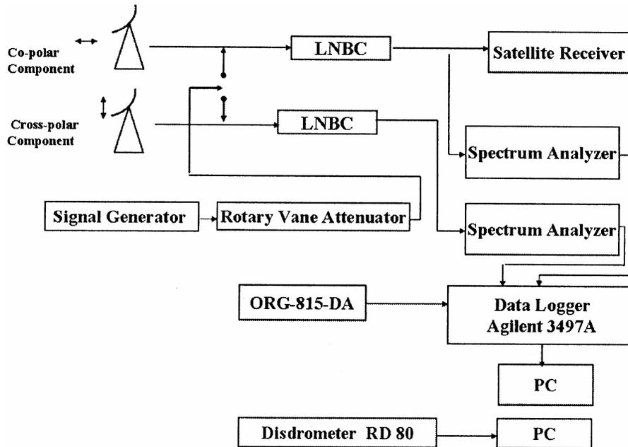
Fig. 1—Experimental set-up for propagation measurements at Ku-band over an earth-space path
