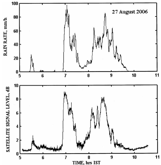
Fig. 2—Typical variation of Ku-band signal level during a rain event
