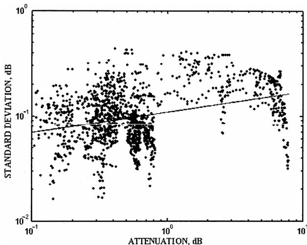
Fig. 9—Variation standard deviation of scintillation against attenuation obtained during the rain event shown Fig. 6. [The solid line is the fitted curve to the data indicating a power-law relationship between the two variables.]
