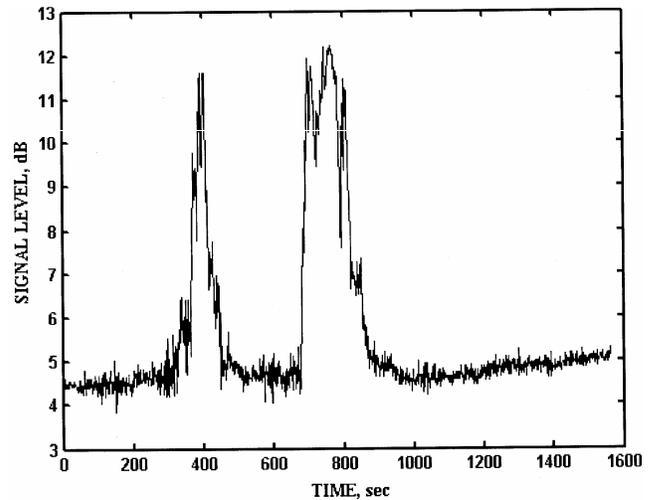
Fig. 6—Typical scintillation of Ku-band satellite signal event associated with rain attenuation.
