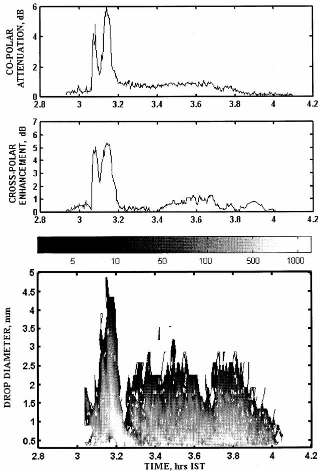
Fig. 5—Temporal variation of the co-polar and cross-polar component of Ku-band satellite signal and drop size distribution during a rain event
