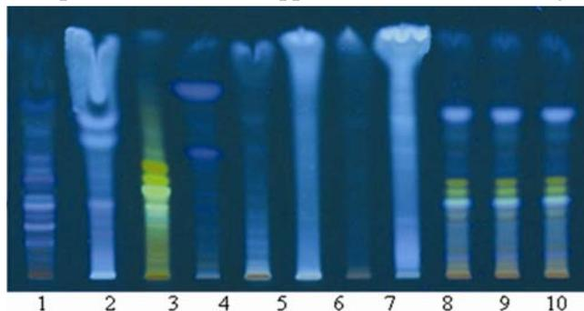
Fig. 4—TLC finger print profile of chloroform fractions and ingredients of Kalyanavleha under UV 366 nm. 1-Glycyrrhiza glabra; 2-Cyclosporum leptophyllum, 3-Curcuma longa, 4-Acorus calamus, 5-Saussurea costus, 6-Piper longum, 7-Zingiber officinalis 8-Cuminum cyminum, 9,10,11-Chloroform fraction of batch I, II and III
