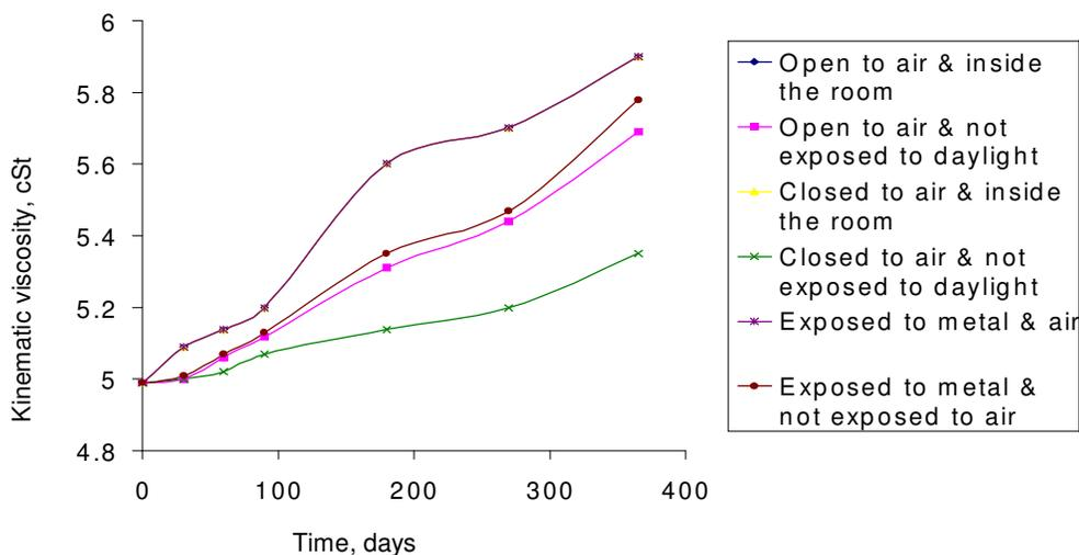
Fig. 2—Viscosity of MOME during storage
