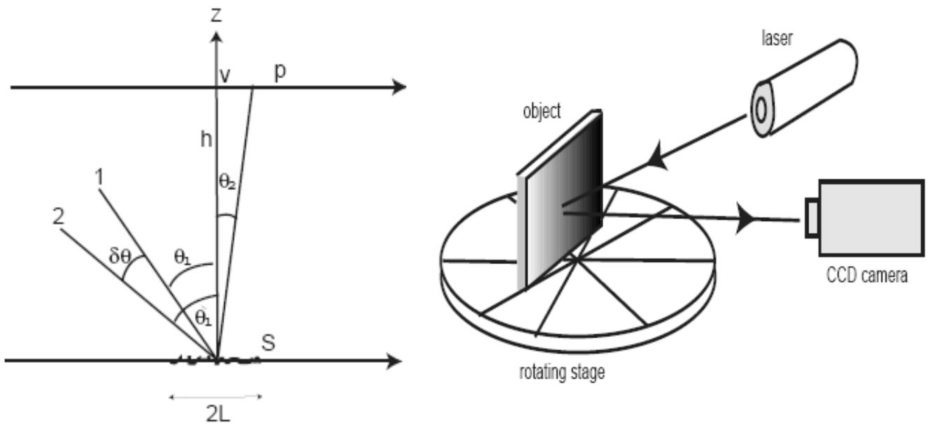
Fig. 4—Geometrical description of angular displacement of specimen
