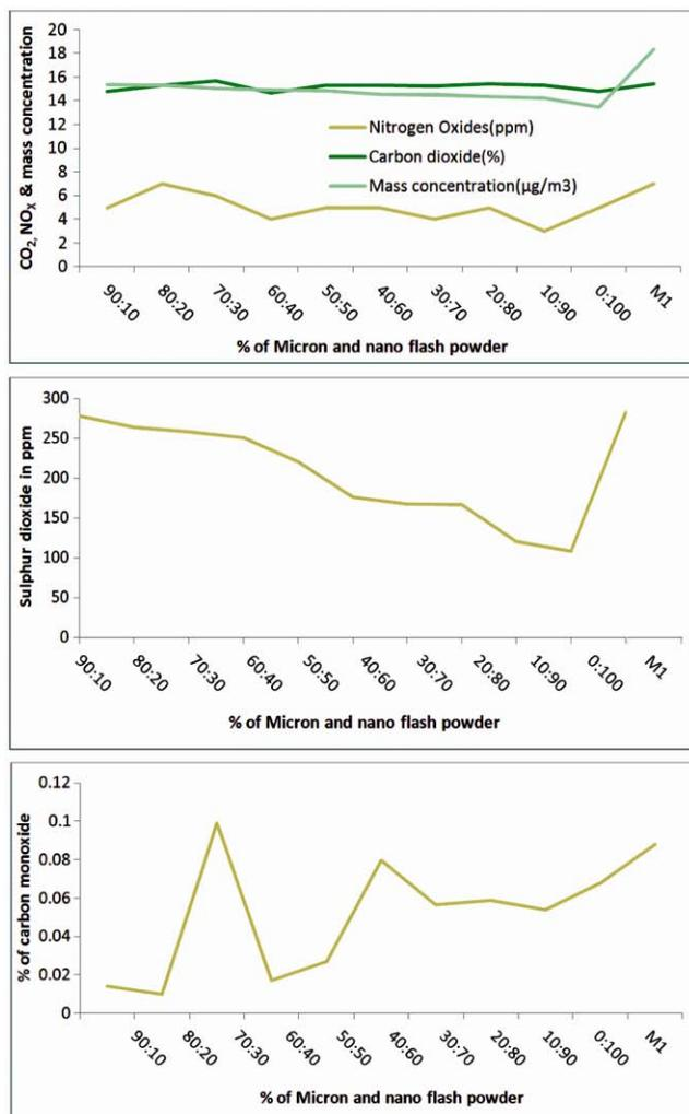
Fig. 1—Gas analysis for the flash powder & suspended particle concentration in air
