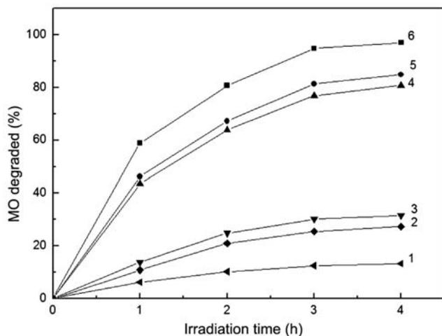
Fig. 5 – Degradation curves of MO with UV light irradiation time. [1, photolysis of MO; 2, ACF in presence of UV light; 3, 0.20 mol% Ce/TiO<sub>2</sub>/ACF in absence of UV light; 4, TiO<sub>2</sub> in presence of UV light; 5, TiO<sub>2</sub>/ACF in presence of UV light; 6, 0.20 mol% Ce/TiO<sub>2</sub>/ACF in presence of UV light].
