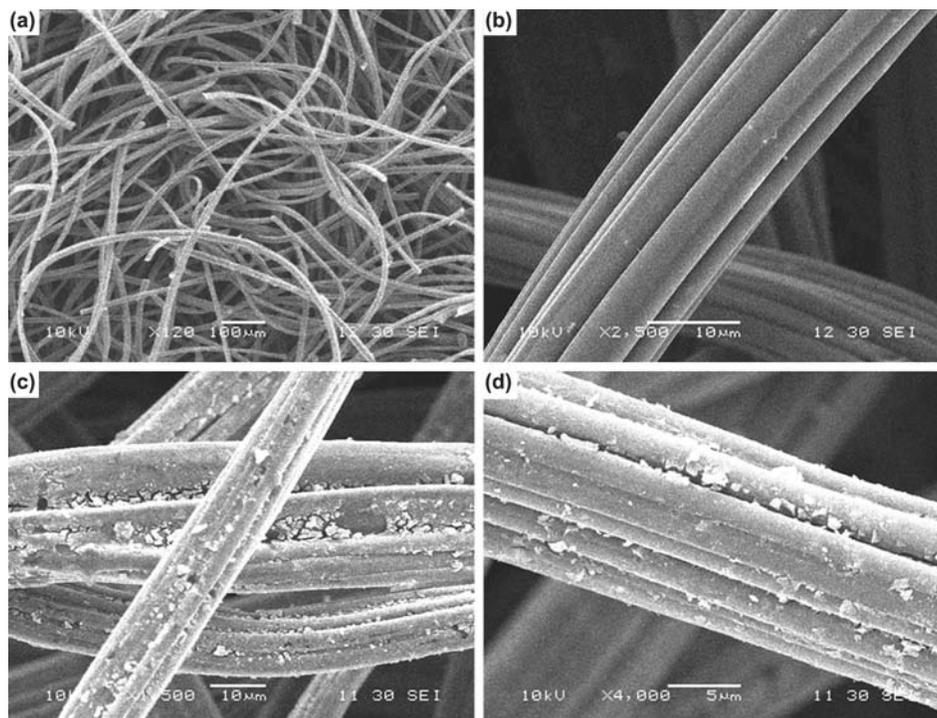
Fig. 1 – SEM photographs of pure ACF and 0.20 mol%Ce/TiO<sub>2</sub>/ACF photocatalyst. [(a) ACF, 120x; (b) ACF, 2500x; (c) Ce/TiO<sub>2</sub> coating on ACF, 1500x; (d) Ce/TiO<sub>2</sub> coating on ACF, 4000x].
