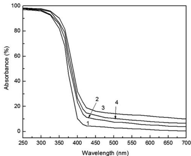
Fig. 3 – UV-vis absorption spectra of catalyst samples. [1, TiO<sub>2</sub>/ACF; 2, 0.10 mol% Ce/TiO<sub>2</sub>/ACF; 3, 0.20 mol% Ce/TiO<sub>2</sub>/ACF; 4, 0.30 mol% Ce/TiO<sub>2</sub>/ACF].
