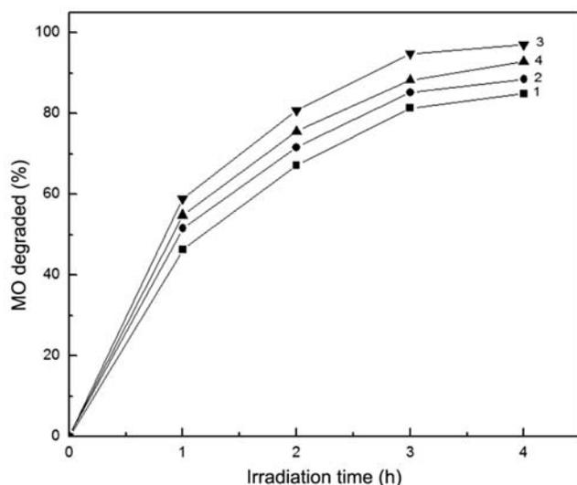
Fig. 4 – Effect of Ce-doped content on the degradation rate of MO. [1, TiO<sub>2</sub>/ACF; 2, 0.10 mol% Ce/TiO<sub>2</sub>/ACF; 3, 0.20 mol% Ce/TiO<sub>2</sub>/ACF; 4, 0.30 mol% Ce/TiO<sub>2</sub>/ACF].
