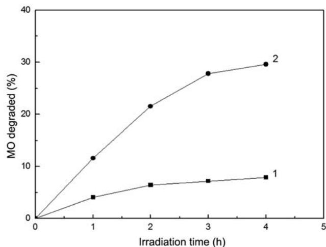
Fig. 6 – Degradation curves of MO with visible light irradiation time. [1, TiO<sub>2</sub>/ACF in presence of visible light; 2, 0.20 mol% Ce/TiO<sub>2</sub>/ACF in presence of visible light].
