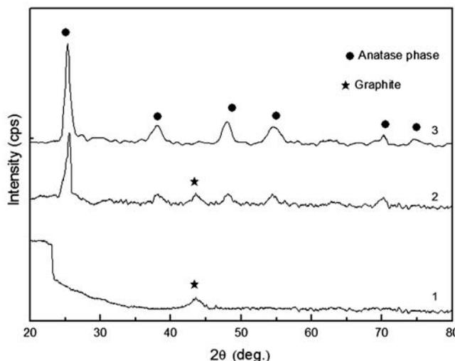
Fig. 2 – XRD patterns of ACF and catalyst samples. [1, ACF; 2, 0.20 mol% Ce/TiO<sub>2</sub>/ACF; 3, TiO<sub>2</sub>].
