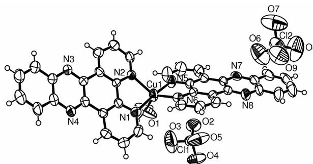
Fig. 1—An ORTEP view of [Cu(dppz)<sub>2</sub>(H<sub>2</sub>O)](ClO<sub>4</sub>)<sub>2</sub> (**1**) showing atom numbering scheme for the metal and hetero atoms and thermal ellipsoids at 50% probability level.
