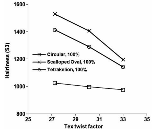
Fig.6—Influence of tex twist factor on hairiness of yarns (S3) corresponding to different cross-sectional shapes of polyester fibre
