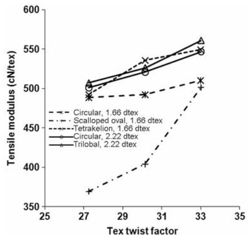
Fig.2—Effect of tex twist factor on tensile modulus of yarns corresponding to different cross-sections of polyester fibre
