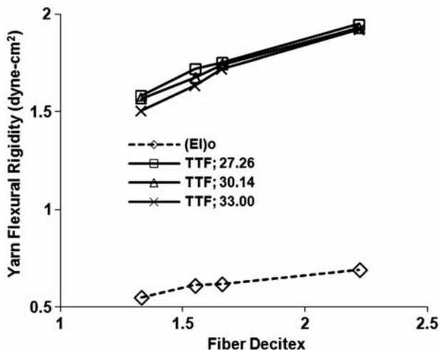
Fig.3—Variation of flexural rigidity of yarns with linear density of polyester fibre under three levels of twist
