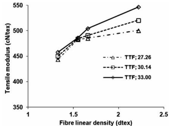
Fig.1—Influence of fibre linear density on tensile modulus of yarns with different levels of twist
