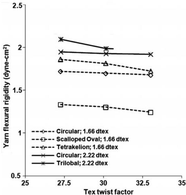
Fig.4—Variation of flexural rigidity of yarns with tex twist factor corresponding to different cross- sections of polyester fibre
