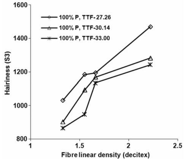
Fig.5—Influence of linear density of polyester fibre on hairiness of yarns (S3) corresponding to three levels of twist
