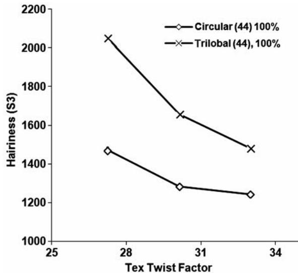
Fig.7—Influence of tex twist factor on hairiness of yarns (S3) corresponding to different cross-sectional shapes of polyester fibre
