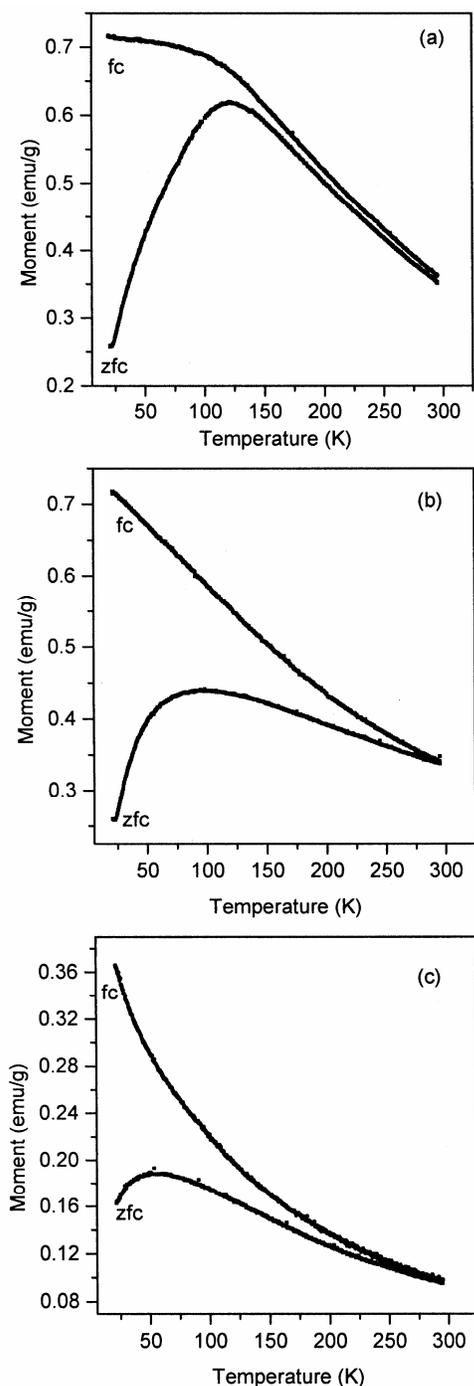
Fig. 4— $M - T$  curves recorded in ZFC and FC modes for the samples (a) Li10 in 8.2 Oe, (b) Li20 in 8.1 Oe and (c) Li30 in 7.8 Oe
