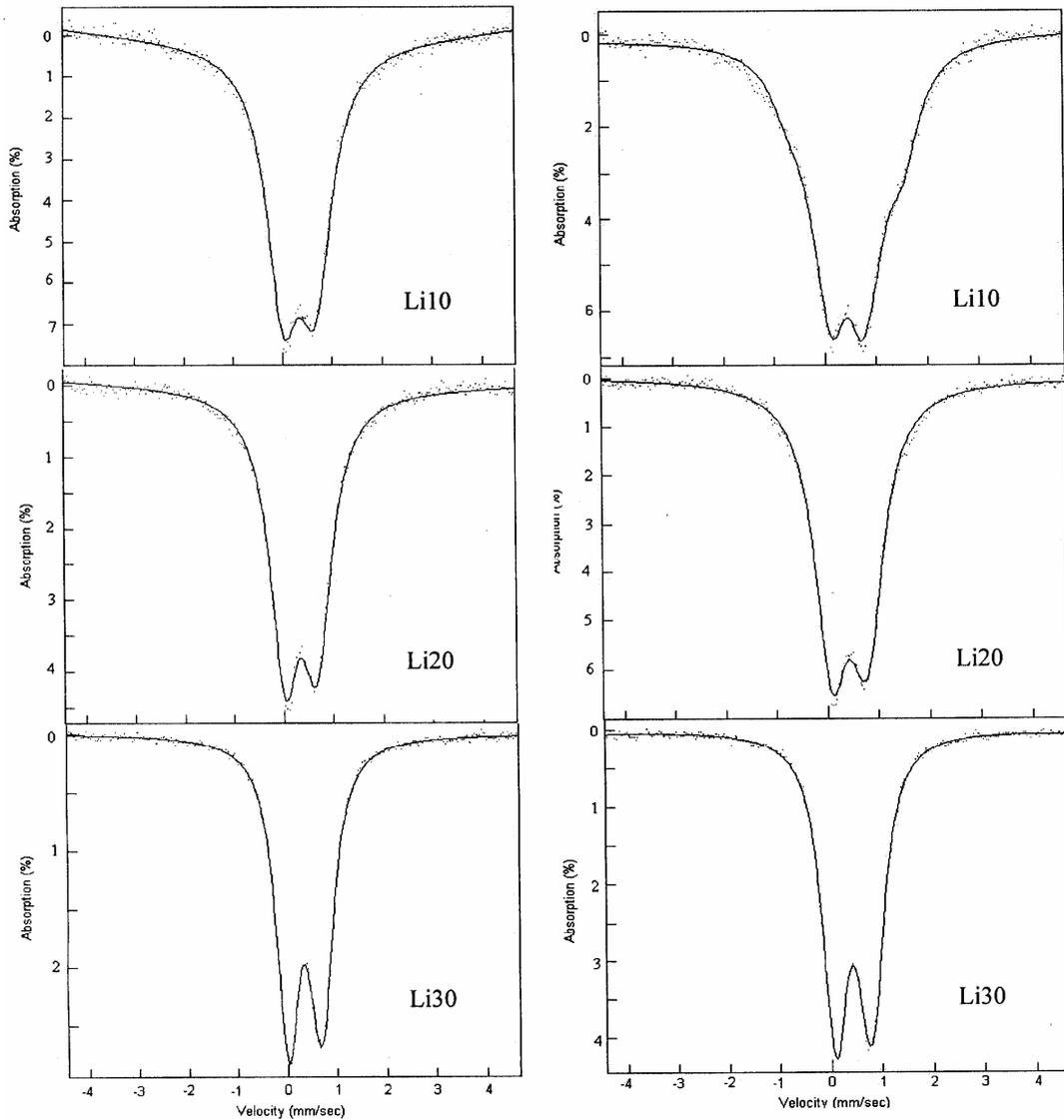
Fig. 5—Mössbauer spectra of the three samples Li10, Li20 and Li30 recorded at (a) 300K and (b) 80K. Fitted envelopes are also shown by continuous lines
