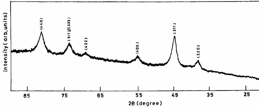
Fig. 1—Fe  $K_{\alpha}$  X-ray powder diffraction pattern recorded at 300K for the sample  $\text{Li}_{0.1}\text{Fe}_{2.9}\text{O}_4$
