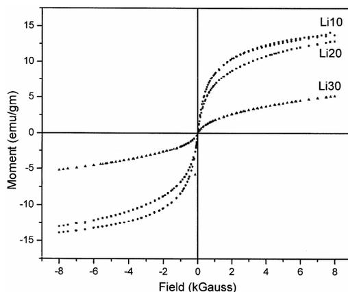
Fig. 3— $M - H$  curves of the three samples Li10, Li20 and Li30 recorded at 300K
