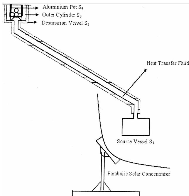
Fig. 1 — Schematic of the inclined heat exchanger unit assisted PSC
