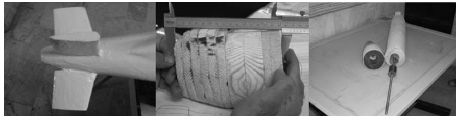
Fig. 8—Construction of Model and Bow of Submarine
