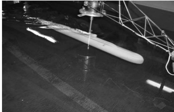
Fig. 9—Submarine Model Test in Towing Tank
