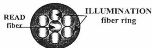
Fig. 3 — Typical fiber bundle arrangement in probe
