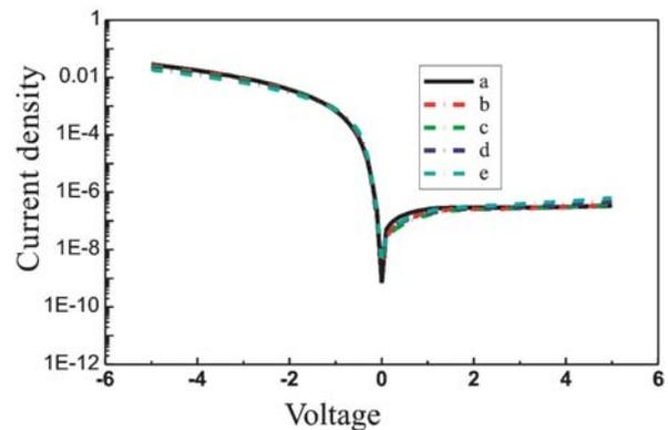
Fig. 4 — Variation of current density with voltage ( $J$ - $V$ ) for Al/PMMA/P-Si/Al structure (a)  $50^{\circ}\text{C}$  ( b)  $75^{\circ}\text{C}$  ( c)  $100^{\circ}\text{C}$  (d)  $125^{\circ}\text{C}$  and ( e)  $150^{\circ}\text{C}$
