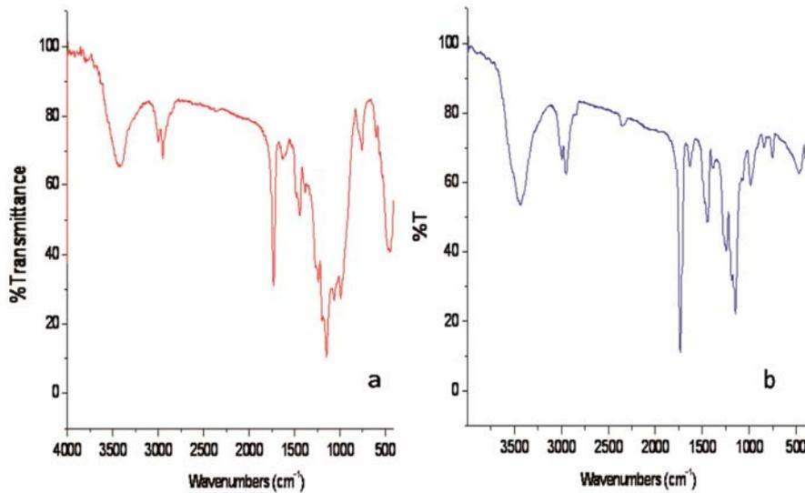
Fig. 1 — FTIR spectrum of PMMA film (a) as grown( $d=160\text{ nm}$ ) (b) annealed at  $100^{\circ}\text{C}$  ( $d=94\text{ nm}$ )
