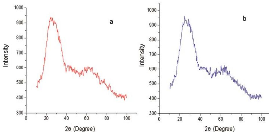
Fig. 2 — XRD pattern of PMMA film (a) as grown( $d=160\text{ nm}$ ) (b) annealed at  $100^{\circ}\text{C}$  ( $d=94\text{ nm}$ )
