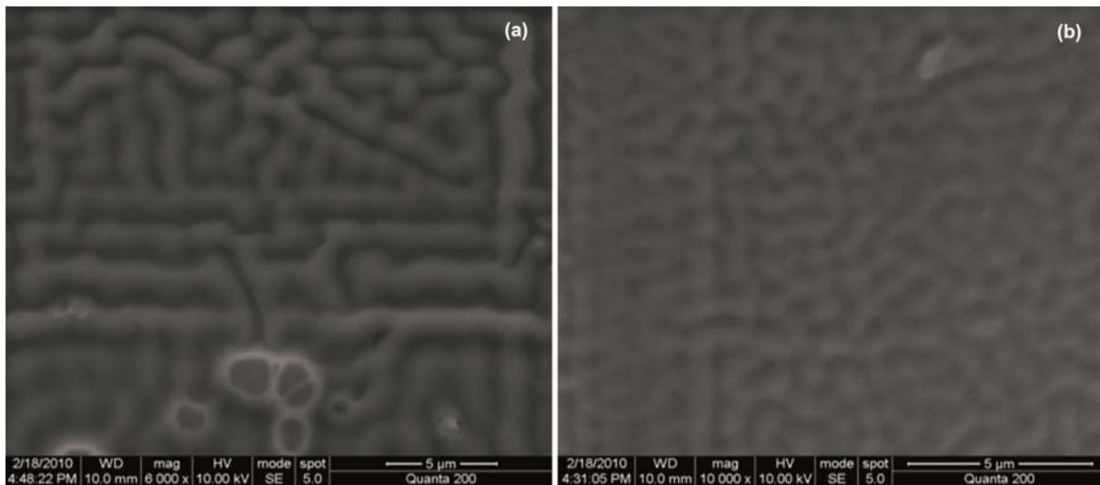
Fig. 3 — SEM images of PMMA film (a) as grown ( $d=160$  nm) (b) annealed at  $100^{\circ}\text{C}$  ( $d=94$  nm)
