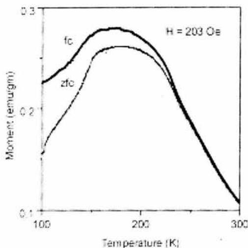
Fig. 4— $M$ - $T$  plot for FMC73 recorded in ZFC and FC modes
