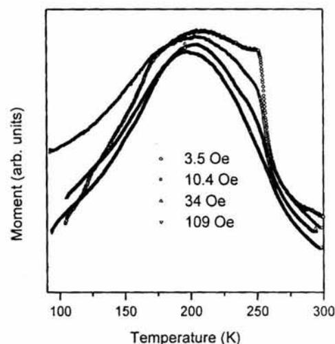
Fig. 2 —  $M$  versus  $T$  plots for FMC55 under different fields
