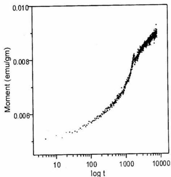
Fig. 5— $M$  versus time plot for FMC55 at 85K in 5.5 Oe after ZFC
