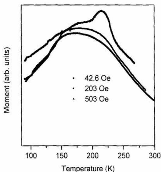
Fig. 3 —  $M$  versus  $T$  plots for FMC73 under different fields
