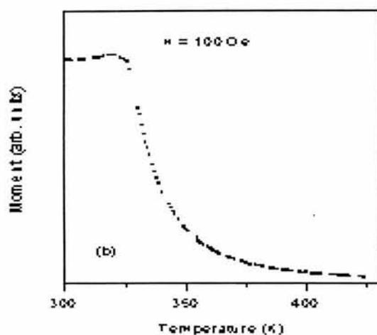
Fig. 1 —  $M$  versus  $T$  plots for FMC37 sample in the temperature range, a) 90 – 300K and b) 300 – 425K
