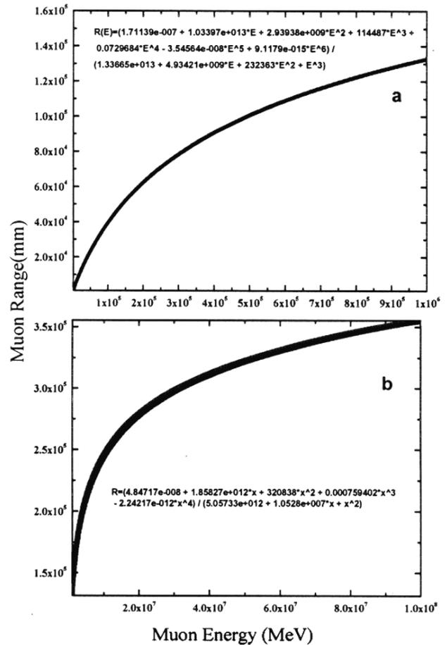
Fig. 2 — Muon range as a function of energy in lead (a) from 1 GeV to 100 GeV (b) from 100 GeV to 100 TeV
