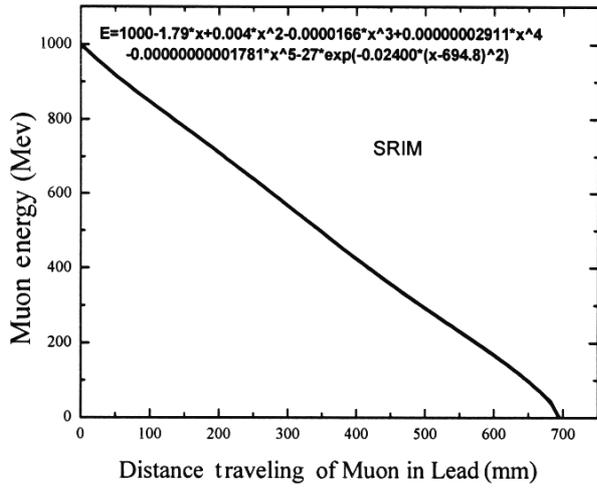
Fig.3 — Muon distance traveled data versus energy in interval 0-1 GeV
