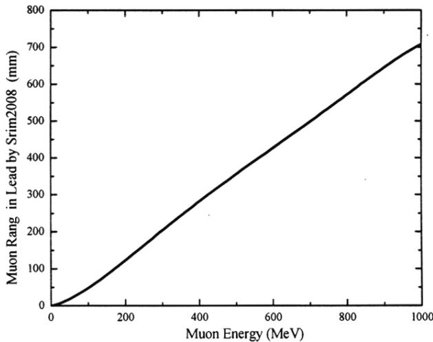
Fig. 1 — Muon range as a function of energy from 0 to 1Gev in lead
