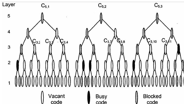
Fig.4 — Illustration of compact code assignment (CCA) scheme
