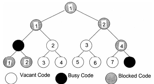
Fig.2 — Four layer code tree with two assigned codes
