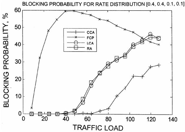
Fig. 6 — Blocking probability versus traffic load for more real time calls
