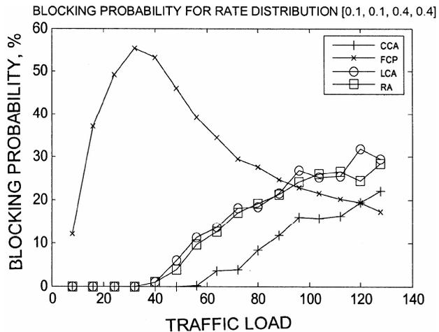
Fig. 7 — Blocking probability versus traffic load for more non-real time calls
