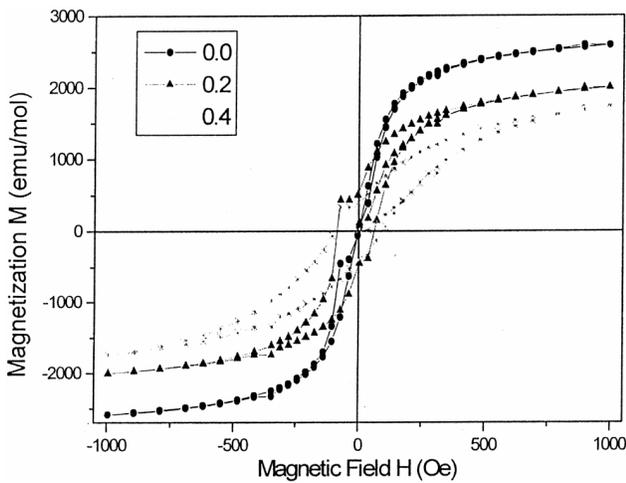
Fig. 4—Field dependence of magnetization curve for ZnAl<sub>x</sub>Fe<sub>2-x</sub>O<sub>4</sub> for x=0.0,0.2,0.4
