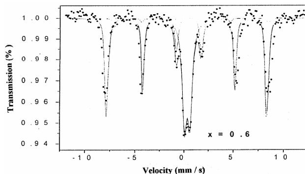
Fig. 7(d)—Mössbauer absorption spectrum at 300K for  $x = 0.6$
