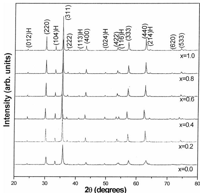
Fig. 1—Typical XRD pattern for  $ZnAl_xFe_{2-x}O_4$  system
