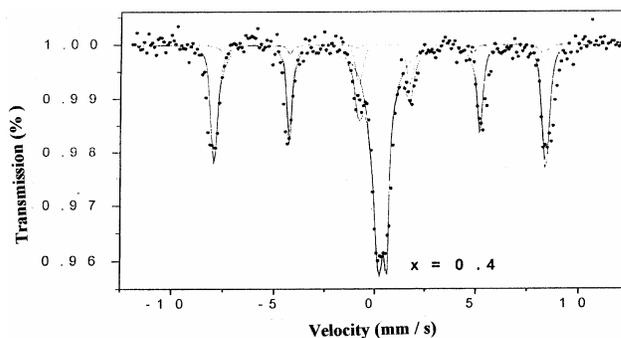
Fig. 7(c)—Mössbauer absorption spectrum at 300K for  $x = 0.4$
