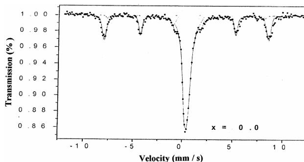
Fig. 7(a)—Mössbauer absorption spectrum at 300K for  $x = 0.0$
