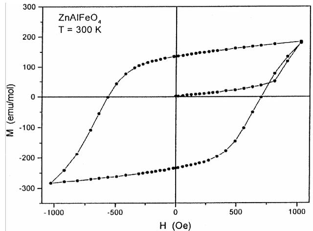
Fig. 6—Field dependence of magnetization curve for ZnAlFeO<sub>4</sub>
