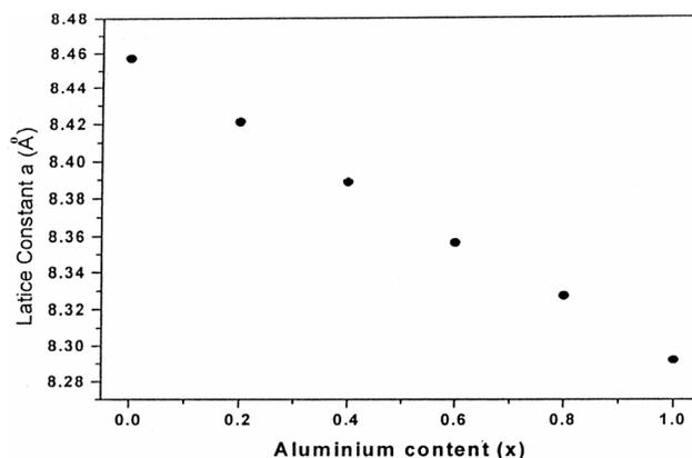
Fig. 2—Variation of lattice constant  $a$  (Å) with aluminium content ( $x$ )
