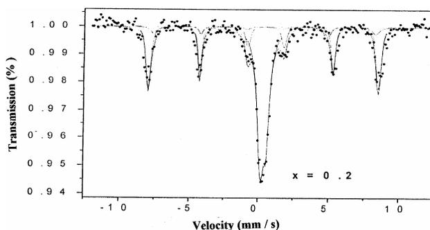
Fig. 7(b)—Mössbauer absorption spectrum at 300K for  $x = 0.2$
