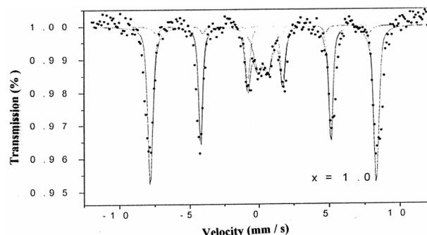
Fig. 7(f)—Mössbauer absorption spectrum at 300K for  $x = 1.0$ Table 2—Hyperfine interaction parameters computed from the Mössbauer absorption spectra recorded at room temperature, isomer shift is given relative to  $\alpha$ -Fe
