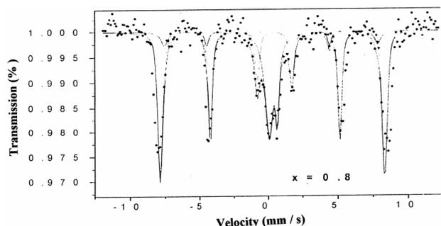
Fig. 7(e)—Mössbauer absorption spectrum at 300K for  $x = 0.8$
