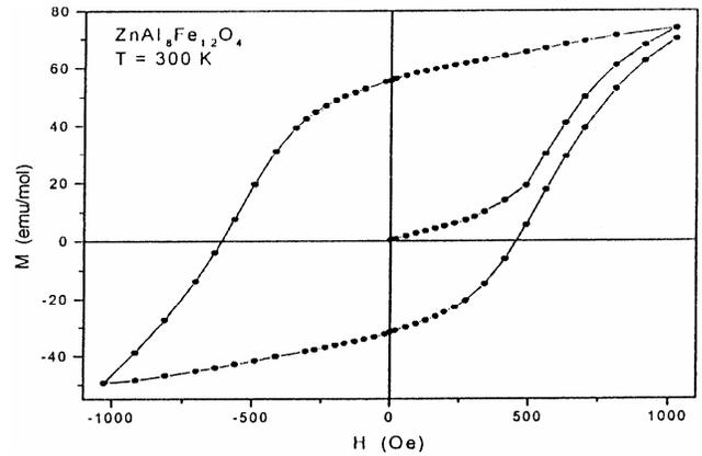
Fig. 5—Field dependence of magnetization curve for ZnAl<sub>0.8</sub>Fe<sub>1.2</sub>O<sub>4</sub>
