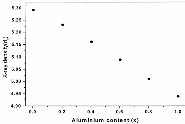
Fig. 3—Variation of X- ray Density with aluminium content (x)
