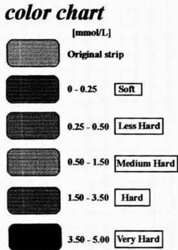
Fig. 1—Colour chart of arsenazo III test strip for water hardness analysis
