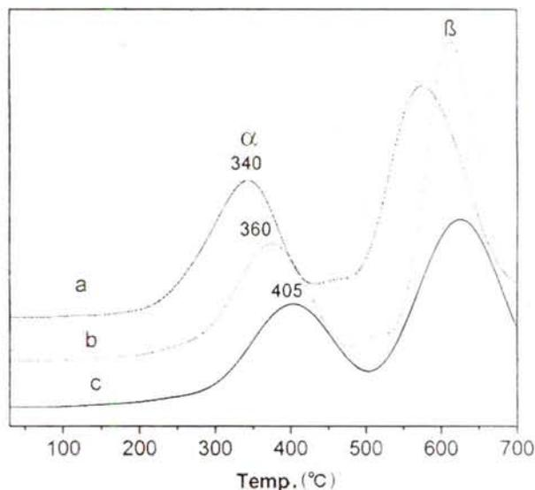
Fig. 3-H<sub>2</sub>-TPR profiles of the La<sub>0.8</sub>Sr<sub>0.2</sub>CoO<sub>3</sub> catalysts prepared by SCS method. [a, alanine; b, glycerol; c, glycine].
