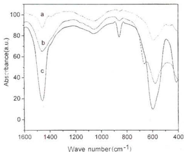
Fig. 2-IR spectra of the La<sub>0.8</sub>Sr<sub>0.2</sub>CoO<sub>3</sub> catalysts prepared by SCS method. [a, alanine; b, glycerol; c, glycine].
