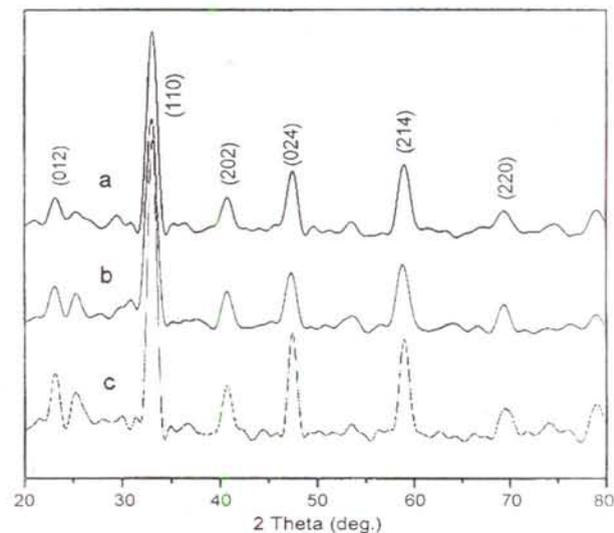
Fig. 1-XRD patterns of the  $\text{La}_{0.8}\text{Sr}_{0.2}\text{CoO}_3$  catalysts prepared by SCS method. [a, alanine; b, glycerol; c, glycine].
