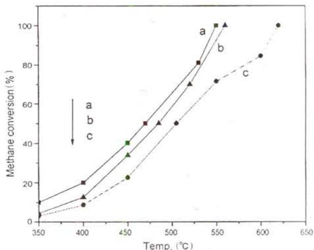
Fig. 4—Catalytic activity profiles of the  $\text{La}_{0.8}\text{Sr}_{0.2}\text{CoO}_3$  catalysts prepared by SCS method. [a, alanine; b, glycerol; c, glycine].
