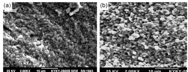
Fig. 4—SEM photographs of discs synthesized from the different raw materials: (a) hydrothermal method; (b) microwave method.
