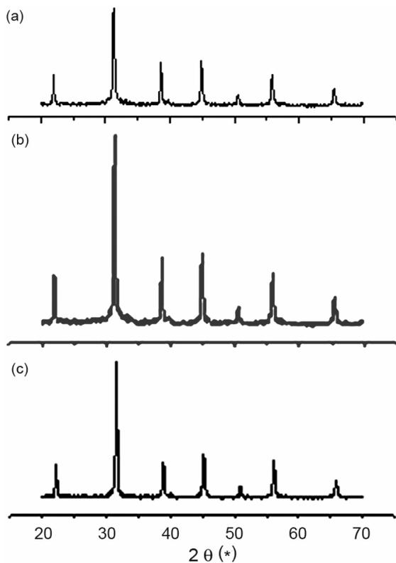
Fig. 1—XRD patterns of nano-BaTiO<sub>3</sub>: (a) Atmospheric liquid-state method; (b) hydrothermal method; and (c) microwave method.
