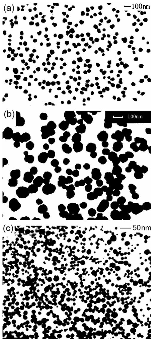
Fig. 2—TEM photographs of nano-BaTiO<sub>3</sub>: (a) atmospheric liquid-state method; (b) hydrothermal method; and, microwave method.
