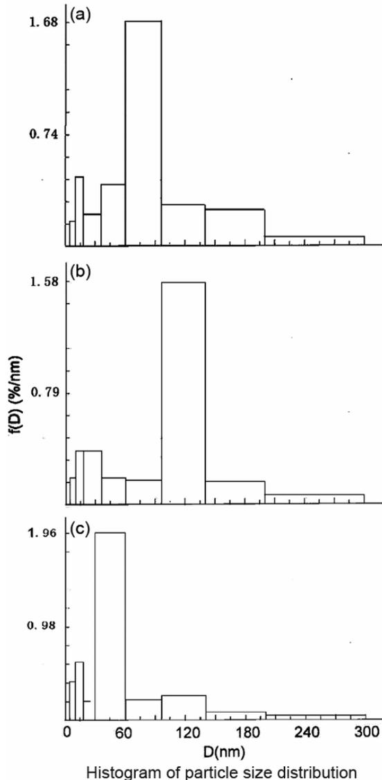
Fig. 3—SAXS patterns of nano-BaTiO<sub>3</sub>: (a) atmospheric liquid-state method; (b) hydrothermal method; and (c) microwave method.
