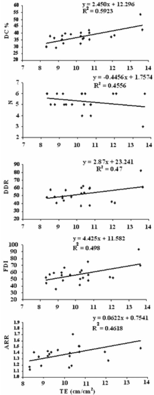
Fig. 5 — Correlation between tensile energy and drape parameters
