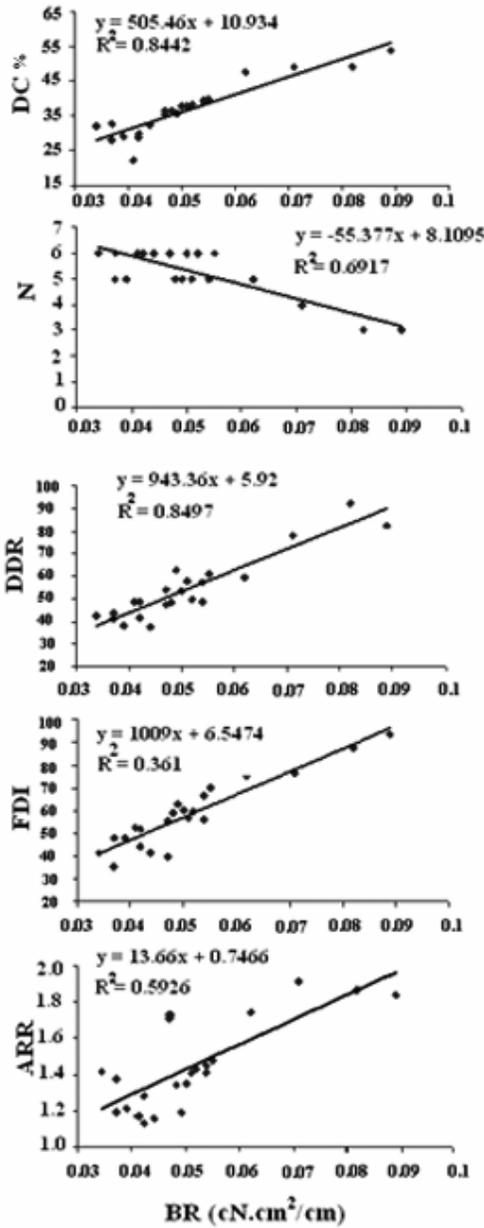
Fig. 4 — Correlation between bending rigidity and drape parameters
