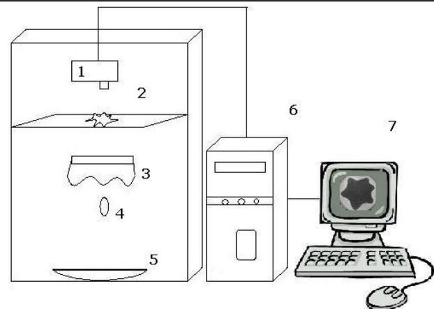
Fig. 1 — Schematic diagram of the digital drapemeter [1-Digital camera, 2-Top glass plate, 3-Bulb, and 6&7- Computer]
