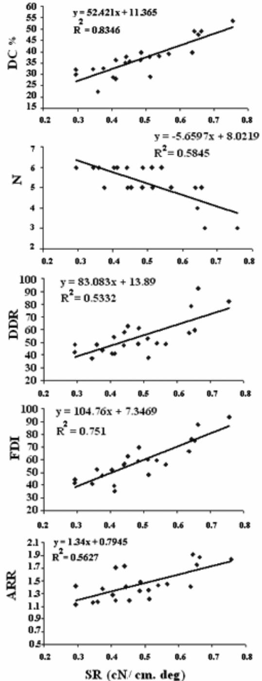
Fig. 7 — Correlation between shear rigidity and drape parameters
