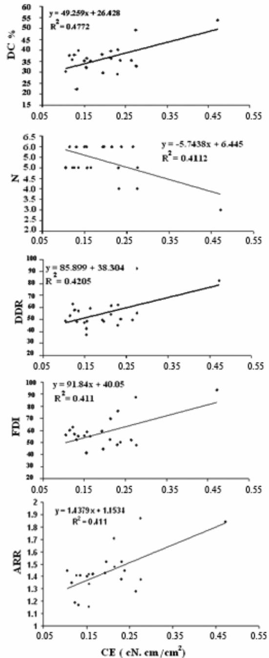
Fig. 8 — Correlation between compressional energy and drape parameters
