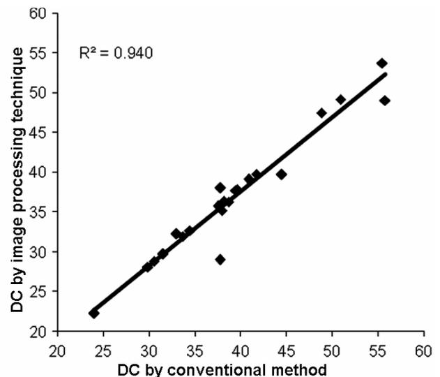
Fig. 3 — Correlation between drape coefficient measured by conventional method and image processing method
