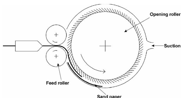
Fig. 1—Schematic diagram of processing propensity tester
