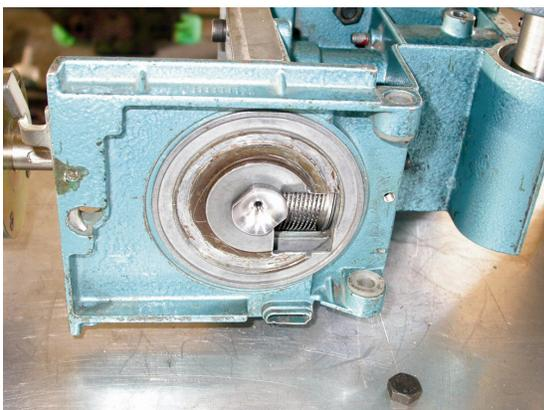
Fig.3 — Magnified view of opening roller (O)
