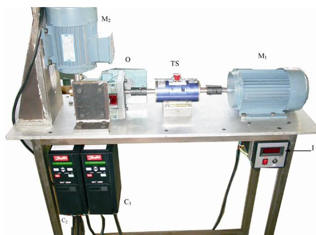
Fig. 2—Fully assembled unit [ $M_1$ —Opening roller drive motor,  $M_2$ —Feed roller drive motor, TS—Torque sensor,  $C_1$  &  $C_2$ —Electronic control panels, I—Indicator, and O—Opening roller]
