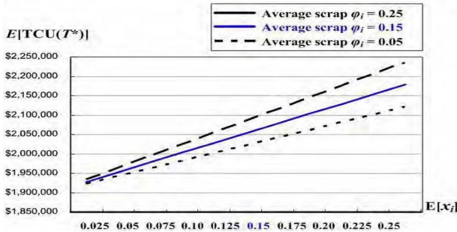
Fig. 36 Variation of average defective rate and average scrap rate effects on the optimal  $E[TCU(T^*)]$  of the proposed multi-item production system
