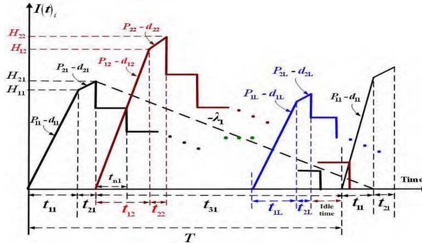
Fig. 16 The on-hand inventory of the perfect quality product  $i$  in the proposed multi-item production system under a common cycle policy
