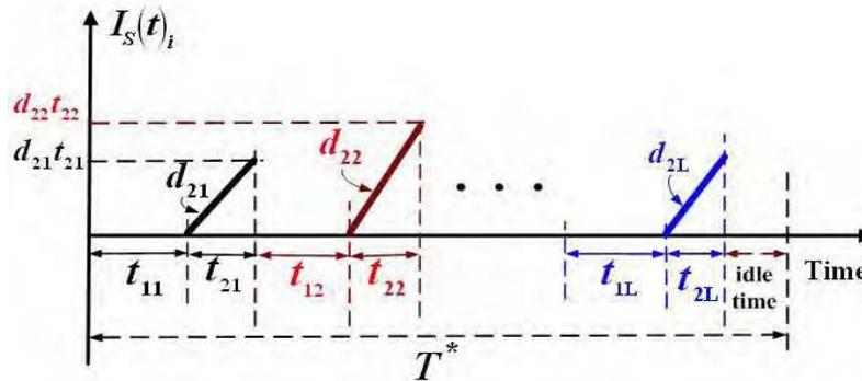
Fig. 26 The on-hand inventory of the scrapped product  $i$  in the proposed multi-item production system under a common cycle policy
