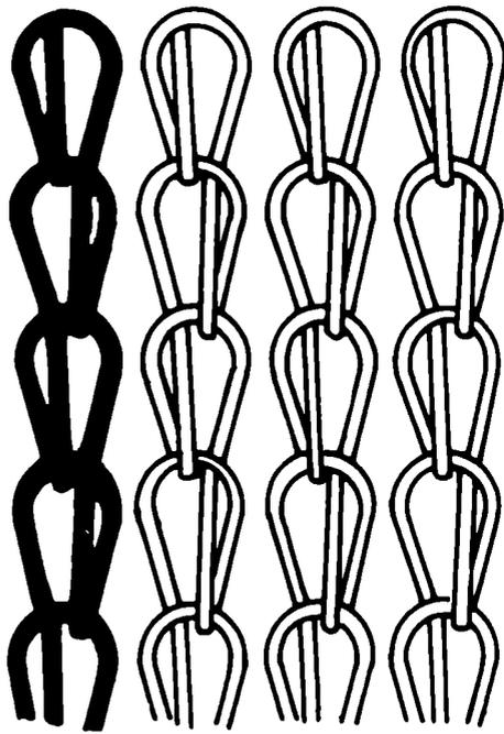
Fig. 3—Pillar stitch for longitudinal stability and/or fabric structure with inlaid weft yarns
