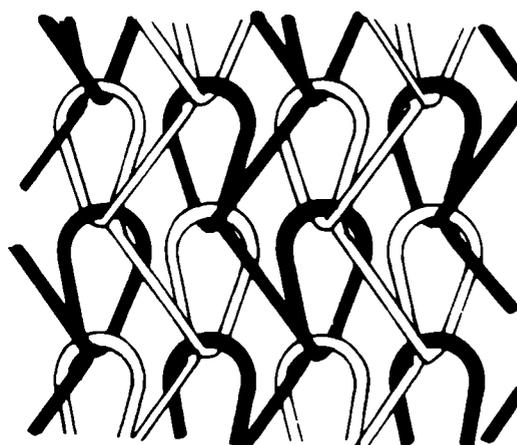
Fig. 2—Tricot: basic stitch structure (1 needle underlap, 1 needle overlap)
