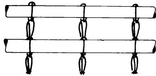
Fig. 4—Monoaxial (unidirectional) DOS with pillar stitches holding inlaid weft yarns
