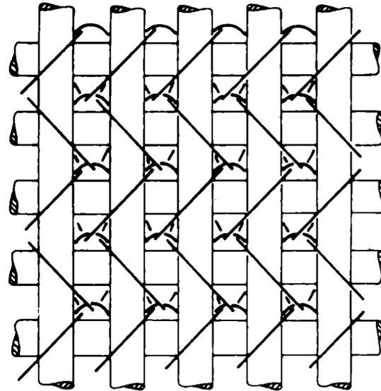
Fig. 5—Perpendicular biaxial DOS—warp and weft yarn layers held by a tricot stitch
