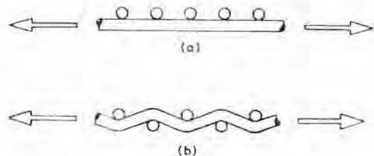
Fig. 8—(a) Woven structure—weft yarn bent due to intertwining with warp yarns; and (b) Warp knit structure—inlaid weft yarn lies absolutely straight
