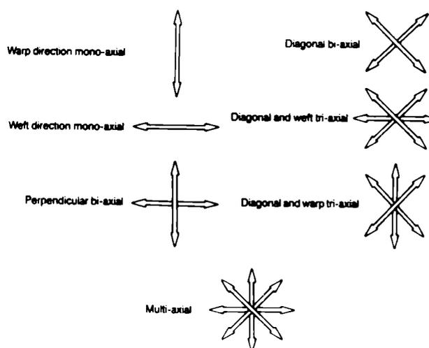
Fig. 1—Schematic diagrams of various directionally-oriented inlay warp structures
