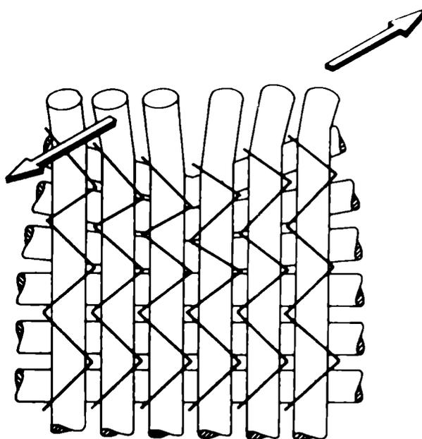
Fig. 9—Biaxial warp inlay DOS under force. "Bunching" phenomenon increases tear resistance
