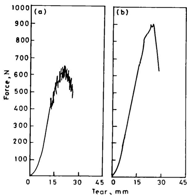
Fig. 10—Trapezoid tear propagation resistance: (a) woven fabric, and (b) multiaxial inlay warp knit fabric (Karl Mayer)
