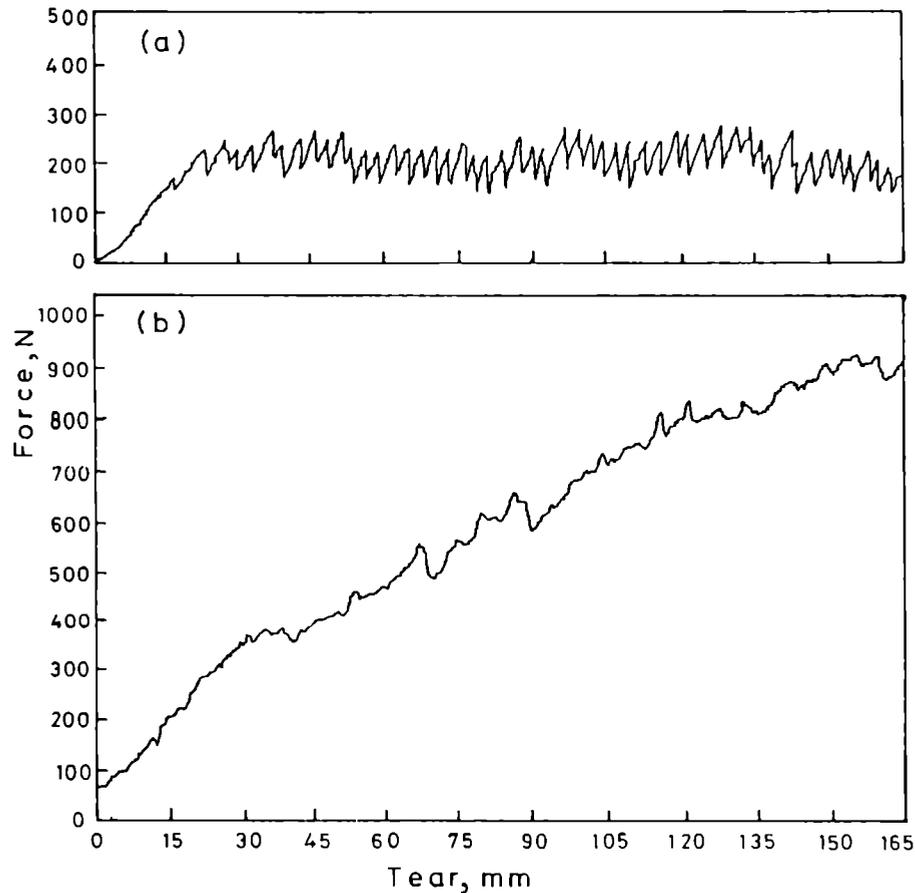
Fig. 11—Shank tear propagation resistance: (a) woven fabric, and (b) multiaxial inlay warp knit fabric (Karl Mayer)
