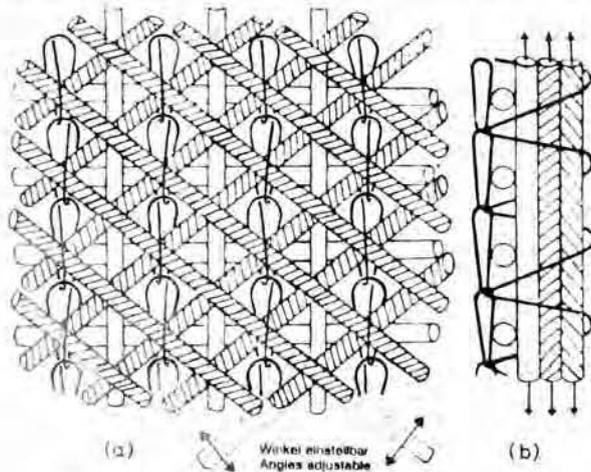
Fig. 6—Multiaxial DOS (Karl Mayer) [a—technical fabric (left side), and b—yarn layers held together by stitching yarn]
