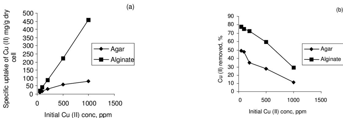
Fig. 3—Effect of initial metal ion concentration on: a) specific uptake of Cu(II) by immobilized biomass; and b) Cu(II) biosorption on immobilized biomass
