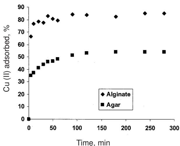
Fig. 4—Effect of incubation time on Cu(II) biosorption by immobilized biomass of *Bacillus cereus* M<sup>16</sup>
