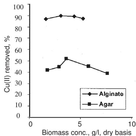
Fig. 2—Effect of biomass concentration on Cu(II) ion biosorption by *Bacillus cereus* M<sup>1</sup><sub>16</sub> biomass immobilized in calcium alginate and agar agar gel
