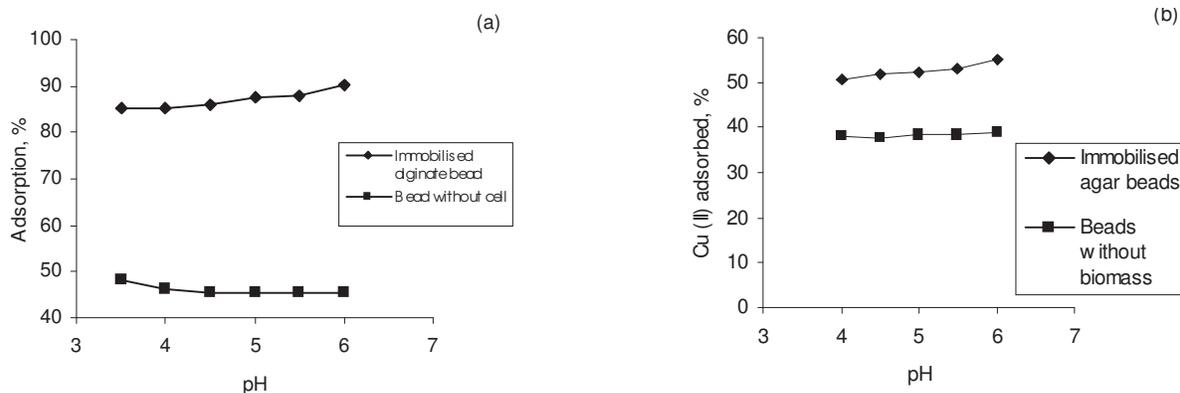
Fig. 1—Effects of initial pH on Cu(II) biosorption : a) Immobilized biomass and calcium alginate bead without biomass; and b) Immobilized biomass and agar agar beads without biomass
