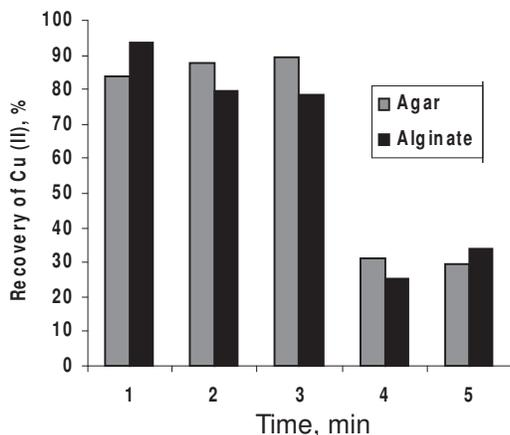
Fig. 6—Desorption capacity of various eluents (HCl-1, HNO<sub>3</sub>-2, H<sub>2</sub>SO<sub>4</sub>-3, CH<sub>3</sub>COOH-4, HCOOH-5)
