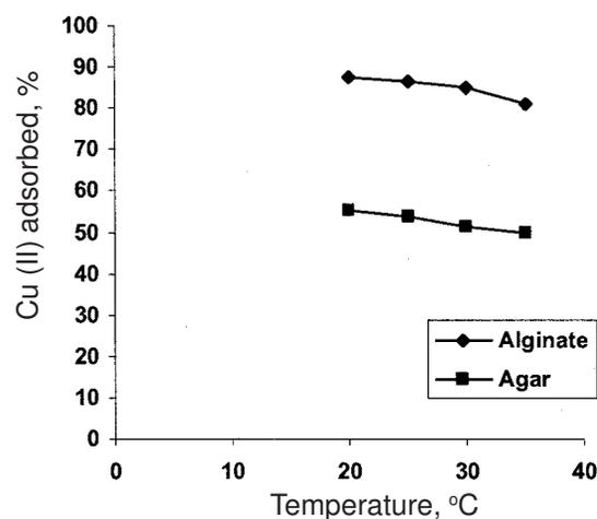
Fig. 5—Effect of temperature on Cu(II) biosorption by *Bacillus cereus* M<sup>16</sup> entrapped in calcium alginate and agar agar gel
