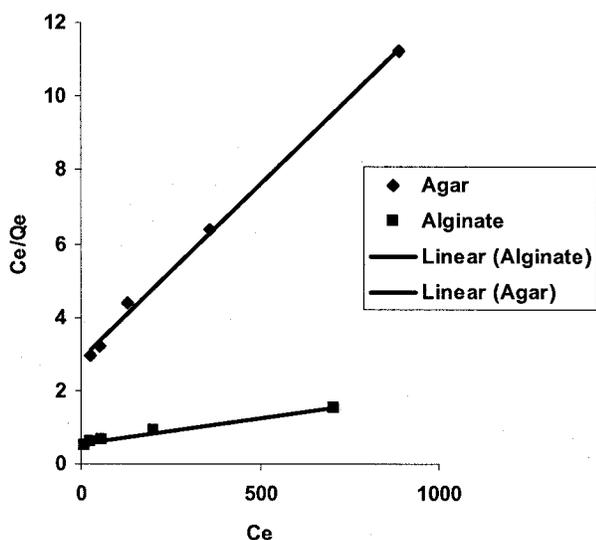
Fig. 8—Langmuir isotherm for biosorption of Cu(II) by *B. cereus* M<sup>1</sup><sub>16</sub> immobilized in calcium alginate gel and agar entrapped *B. Cereus* M<sup>1</sup><sub>16</sub>
