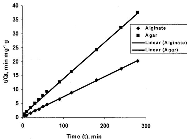
Fig. 9—Pseudo second order adsorption kinetics of Cu(II) on agar immobilized biomass and calcium alginate entrapped biomass
