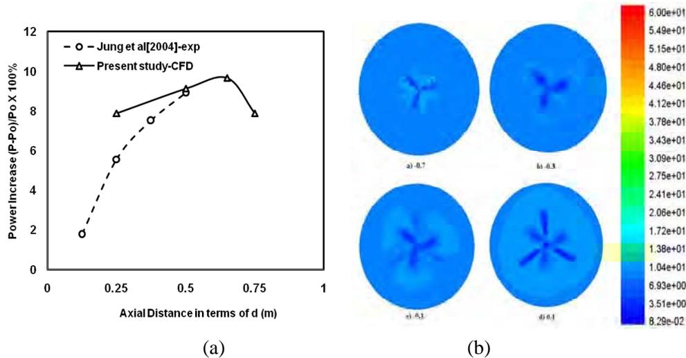
Fig. 3—(a) Comparison of power increase  $((P-P_0)/P_0 \times 100\%)$  and (b) Typical contours of axial velocities for various x/d locations for wind speed of 10 m/s [P is the power of the CFD model and  $P_0$  is the power without considering the wake effects ]
