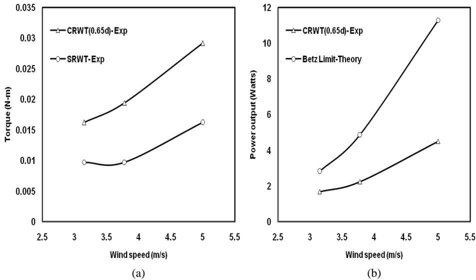
Fig. 6—(a) Variation of torque b) Comparison of power output for CRWT
