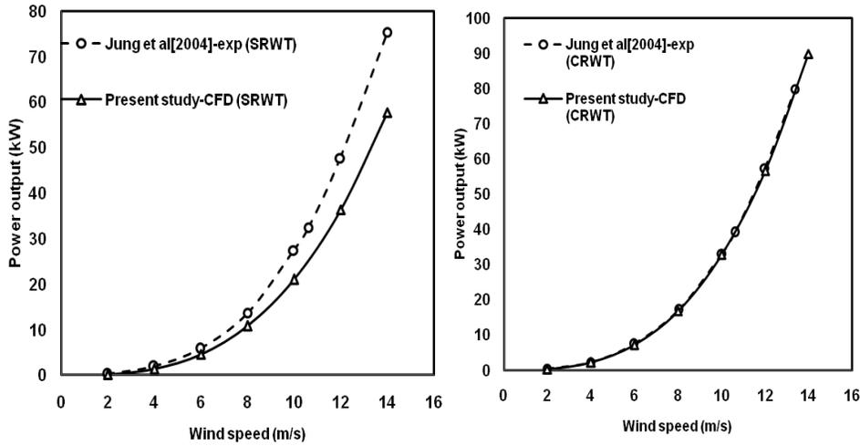
Fig. 5—Comparison of power output for SRWT & CRWT
