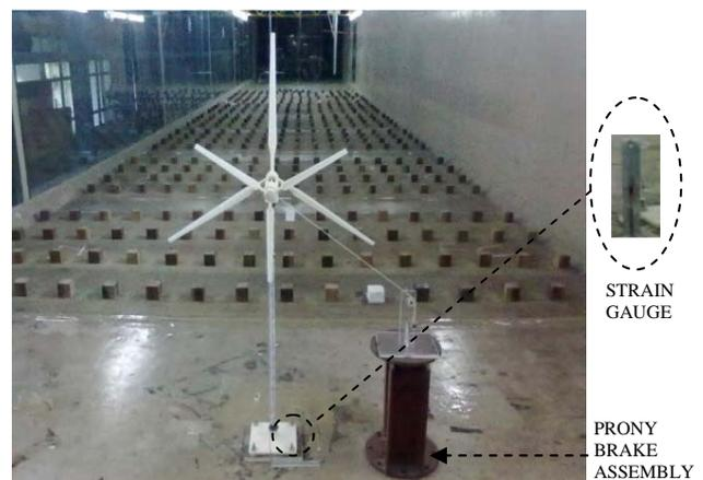
Fig. 2—Experimental setup of CRWT model with prony brake assembly
