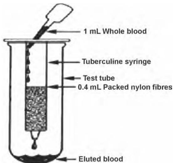
Figure 1— Schematic representation of packed nylon column
