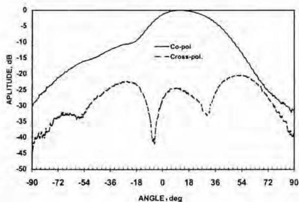
Fig. 4—Measured radiation pattern in azimuth plane at port for vertical polarization at 5.3 GHz.
