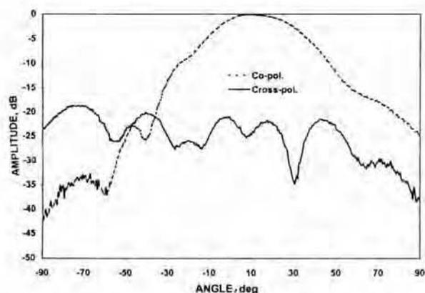
Fig. 3—Measured radiation pattern in elevation plane at port for horizontal polarization at 5.3 GHz
