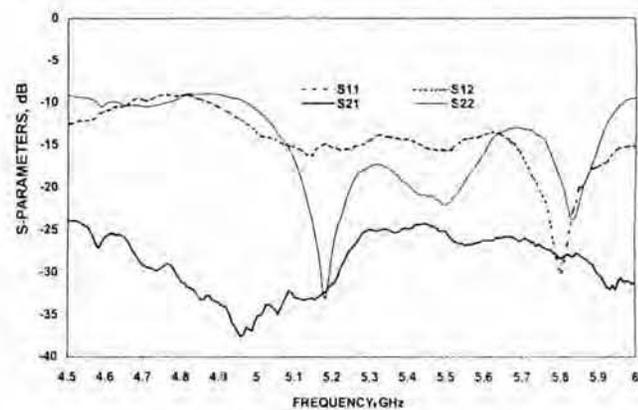
Fig. 2—Measured S-parameters (The data for curves S<sub>12</sub> and S<sub>21</sub> are almost identical and very difficult to demark the two.)
