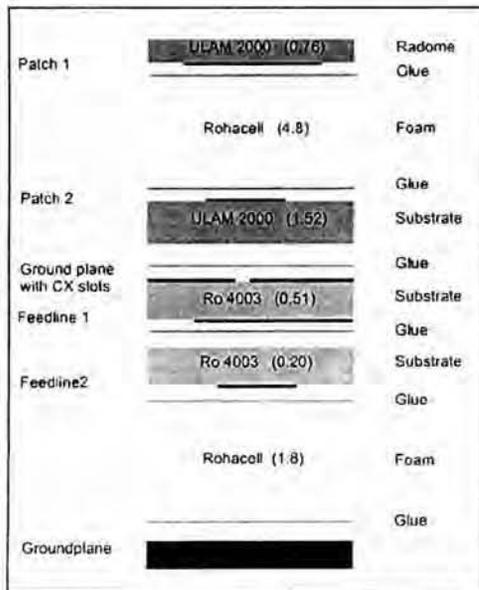
Fig.1—Stacked patch antenna with different layered substrates and thickness used as radiating element (The number in the parentheses represents the thickness in mm)
