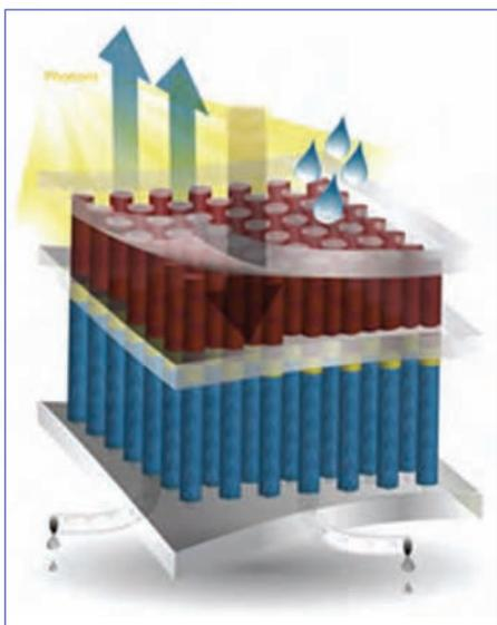
Conceptual drawing of an artificial photosynthetic system that uses only light, water, and carbon dioxide as inputs, and produces clean, renewable fuel.
