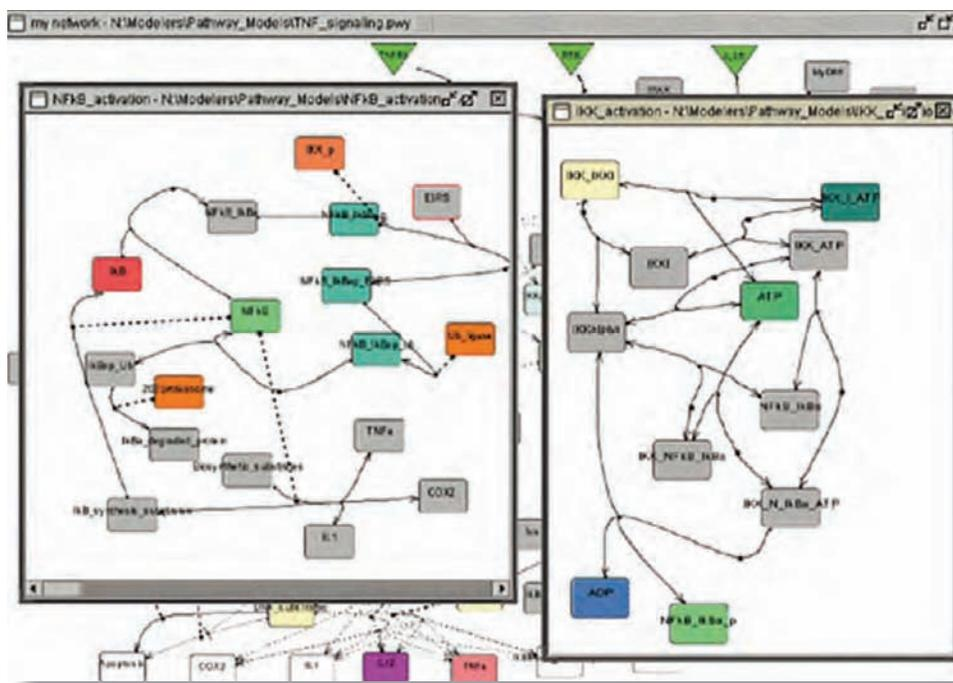
The screen shots in the image from software application PathwayPrism showing the representation of the signalling modules nuclear factor-B (NF- B) and inhibitor of NF- B kinase (IKK) within the larger pathway of the signal-transduction processes that are involved in stress signalling. This representation is converted into a set of mathematical relationships that can be simulated to understand complex cell behaviour.
