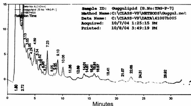
Fig. 2 — HPLC with retention times for a sample in a batch of *Yogaraja guggulu*
