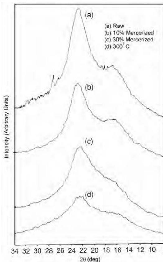
Fig. 3—Variation in XRD profiles with concentration of mercerization and temperature
