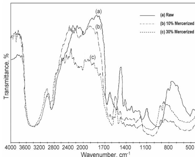
Fig. 2—Variation in IR absorption bands with concentration of mercerization
