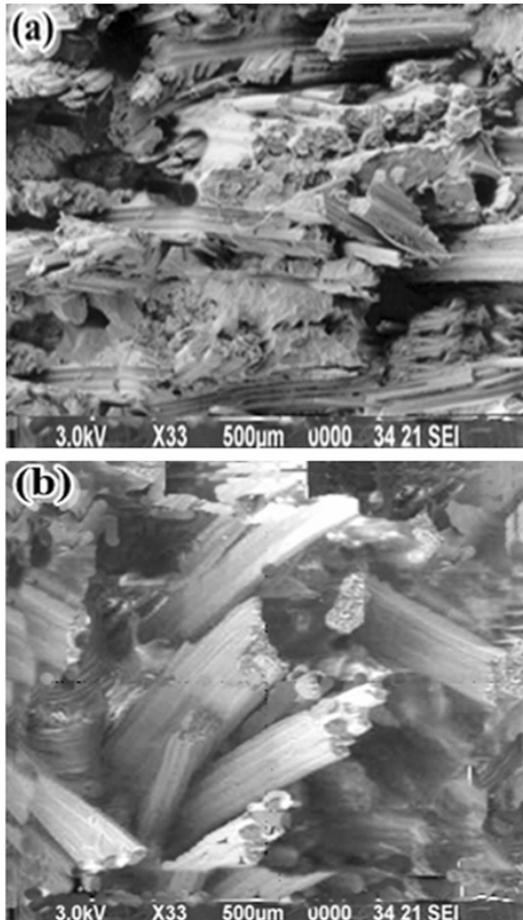
Fig. 2— SEM picture of impact fracture surface of composite board made with (a) high temperature, pressure and time, and (b) low temperature, time and moderate pressure
