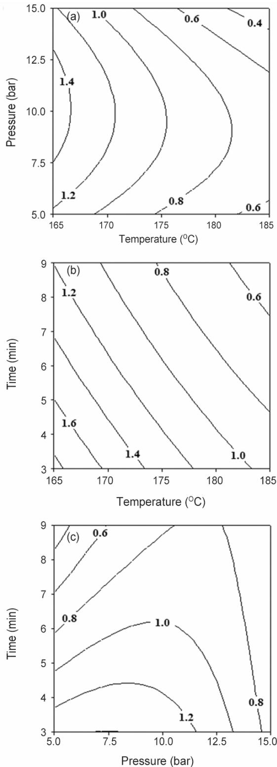
Fig. 1 —Contour diagrams of impact strength vs. (a) pressure and temperature (hold value: time 6 min), (b) time and temperature (hold value: pressure 10 bar), (c) time and pressure (hold value: temperature 165°C)
