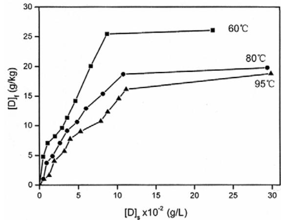
Fig. 1-Adsorption isotherm of berberine on silk
