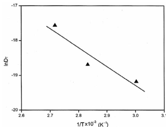
Fig.6–Relationship between  $\ln D_T$  and  $1/T$  for activation energy
