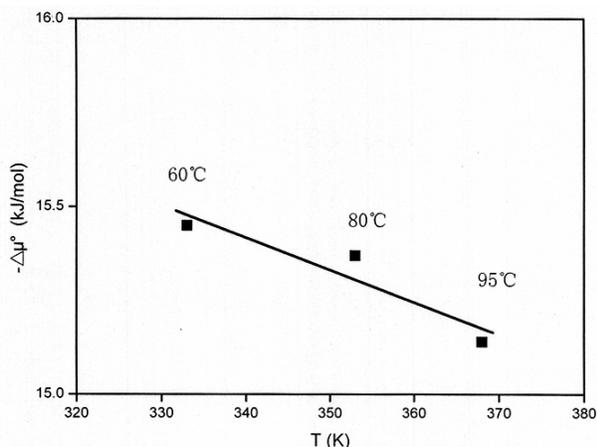
Fig. 3–Relationship between  $-\Delta\mu^\circ$  and  $T$  for silk dyeing with berberine
